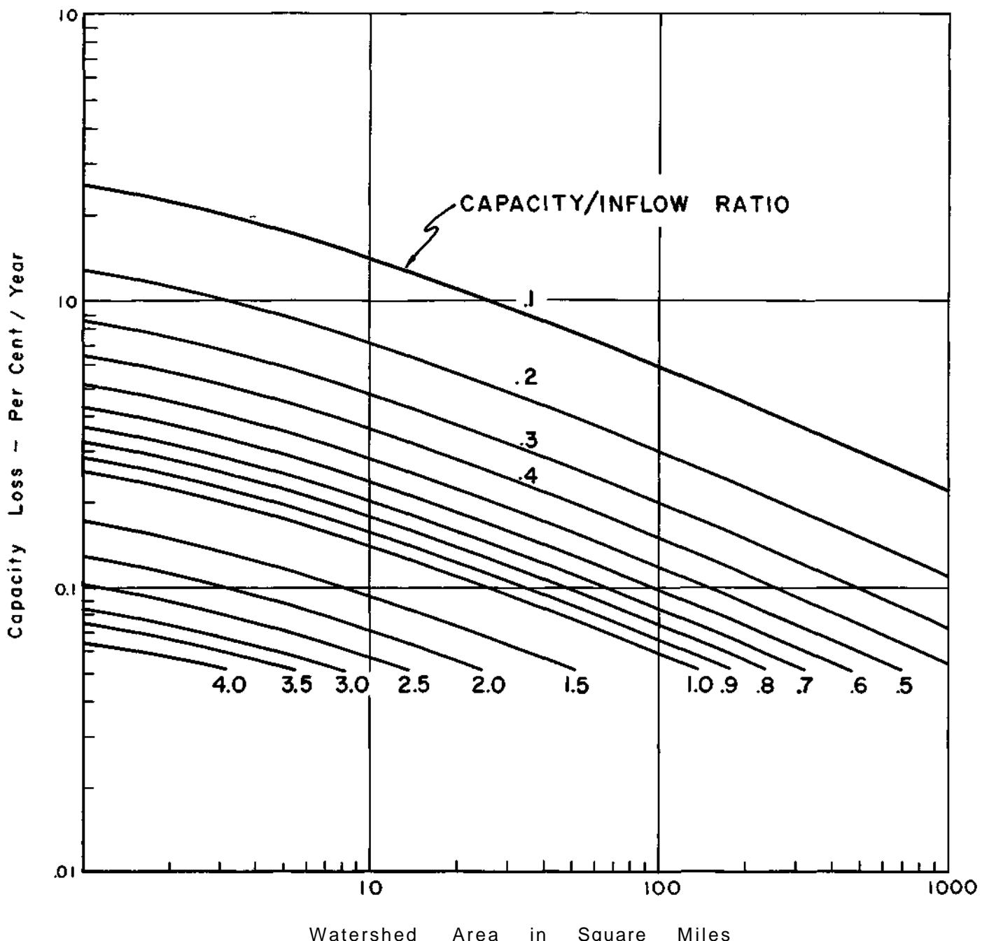
FIGURE 4 RESERVOIR SEDIMENTATION IN SOUTHERN ILLINOIS
