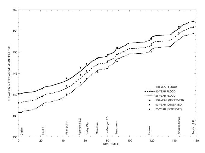
Figure 6. Simulated flood profiles for the Lower Illinois River with flood elevations for 25-, 50-, and 100-year flood events (4%, 2%, and 1% exceedence probability, respectively).
