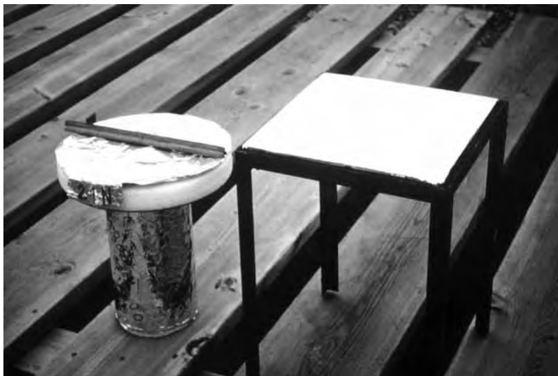
Two hail sensors. On the left is a hail stool and on the right is a hailpad. The hailpad is a 1-square foot piece of styrofoam wrapped in aluminum foil and supported on a stand made of angle-iron.
