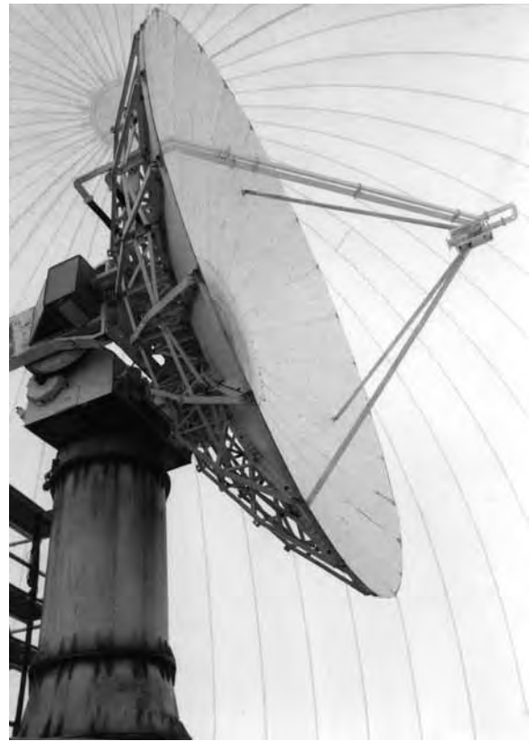
The antenna of the dual-wavelength radar designed and operated by the Illinois State Water Survey to detect hailstones aloft.
