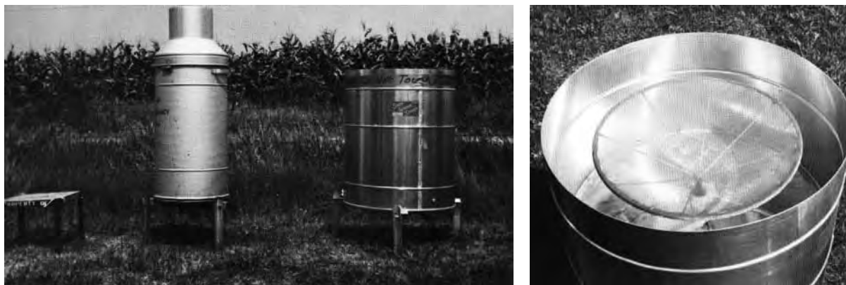
In the left photo is a hailpad, a recording rain gauge, and a recording hail gauge. In the right photo is the sensing platform inside the recording hail gauge, a device designed and developed by the Water Survey.
