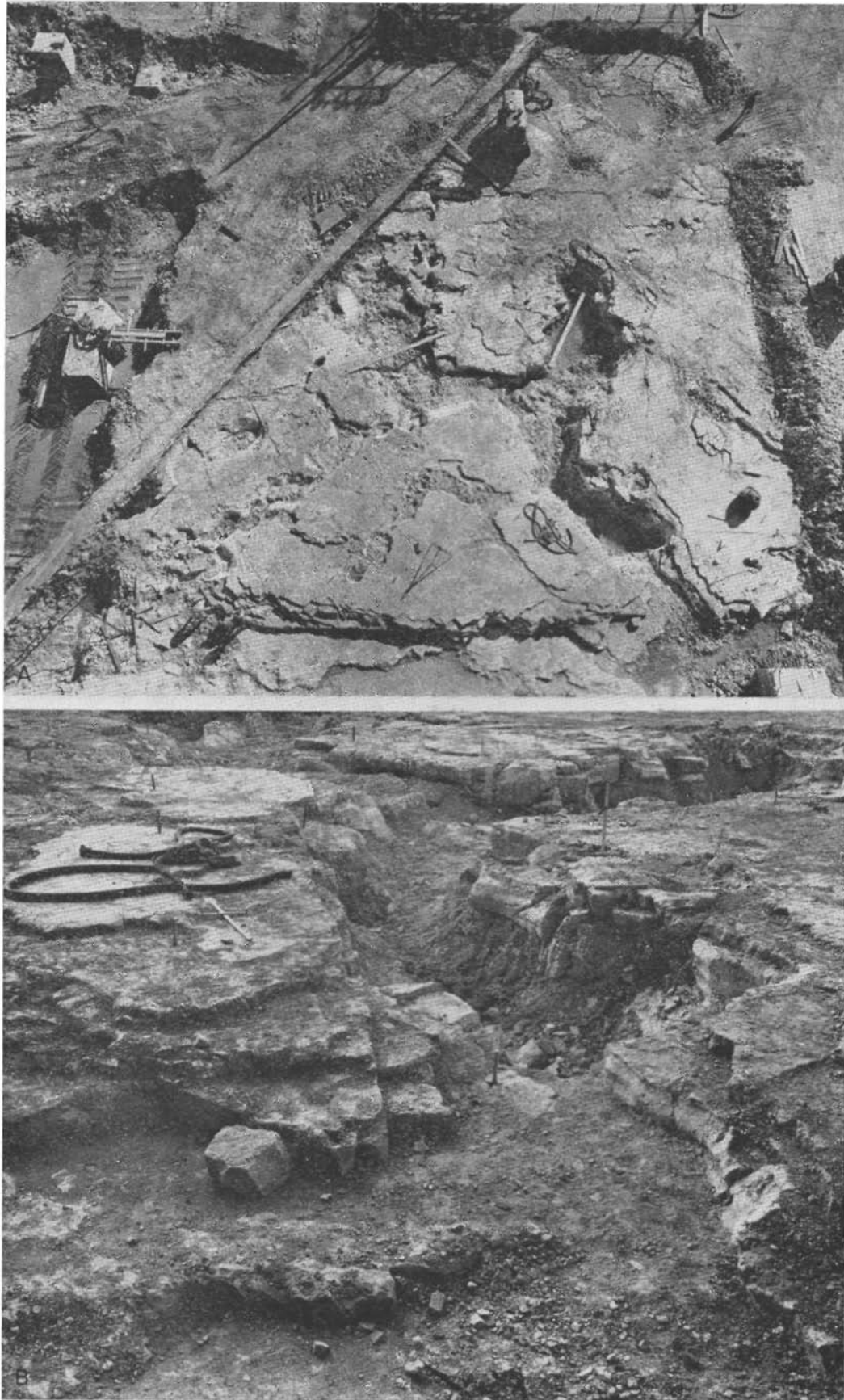
Fig. 17. Aerial and ground views of joint-controlled solution cavities in the Silurian dolomite aquifer (photographs courtesy of the Commonwealth Edison Company).
