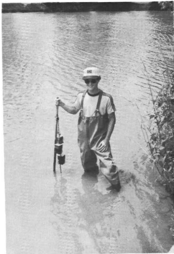
Figure 16. Arrangement of artificial substrates at sampling stations
