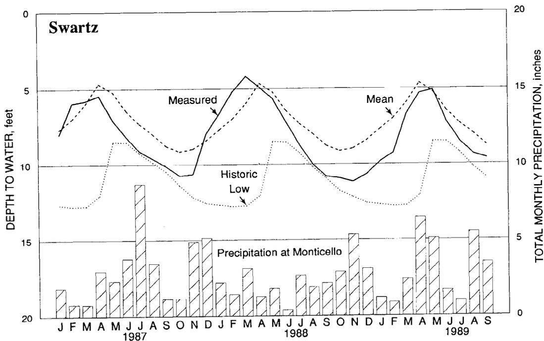
Figure 6.1. Shallow ground-water levels at the Swartz observation well, Piatt County (eastern crop reporting district), and precipitation for nearby Monticello, January 1987 - September 1989
