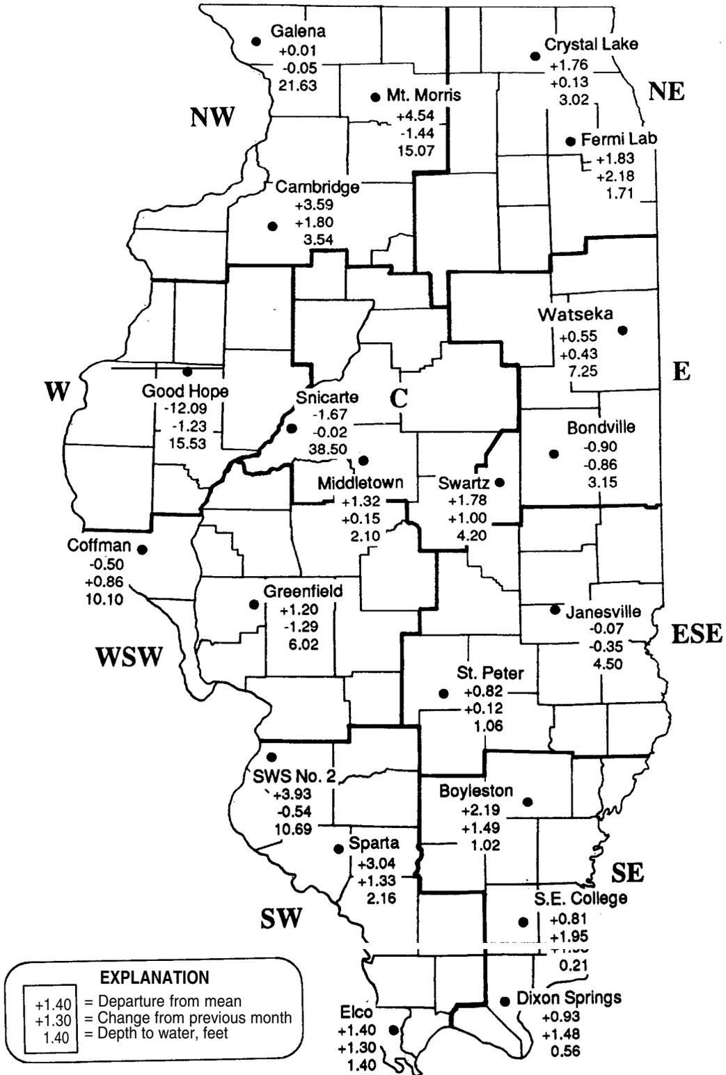
Figure 6.5. Recorded month-end water levels (depth to water), changes from previous month, and departures from mean month-end water levels, March 1988
