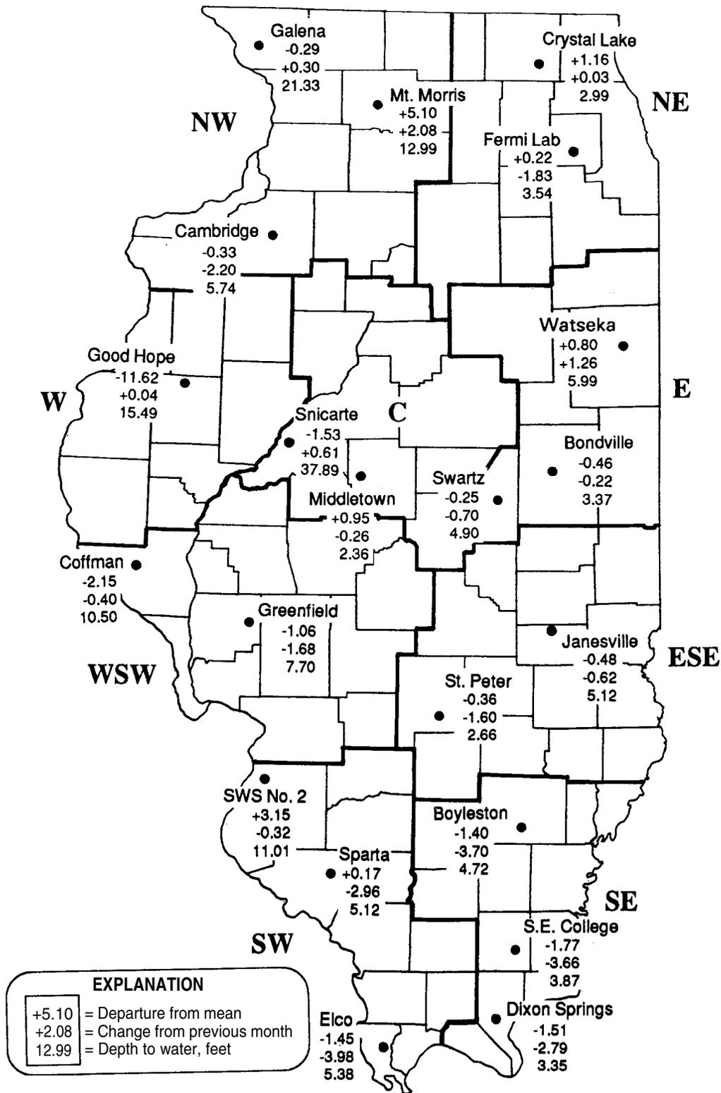
Figure 6.6. Recorded month-end water levels (depth to water), changes from previous month, and departures from mean month-end water levels, April 1988
