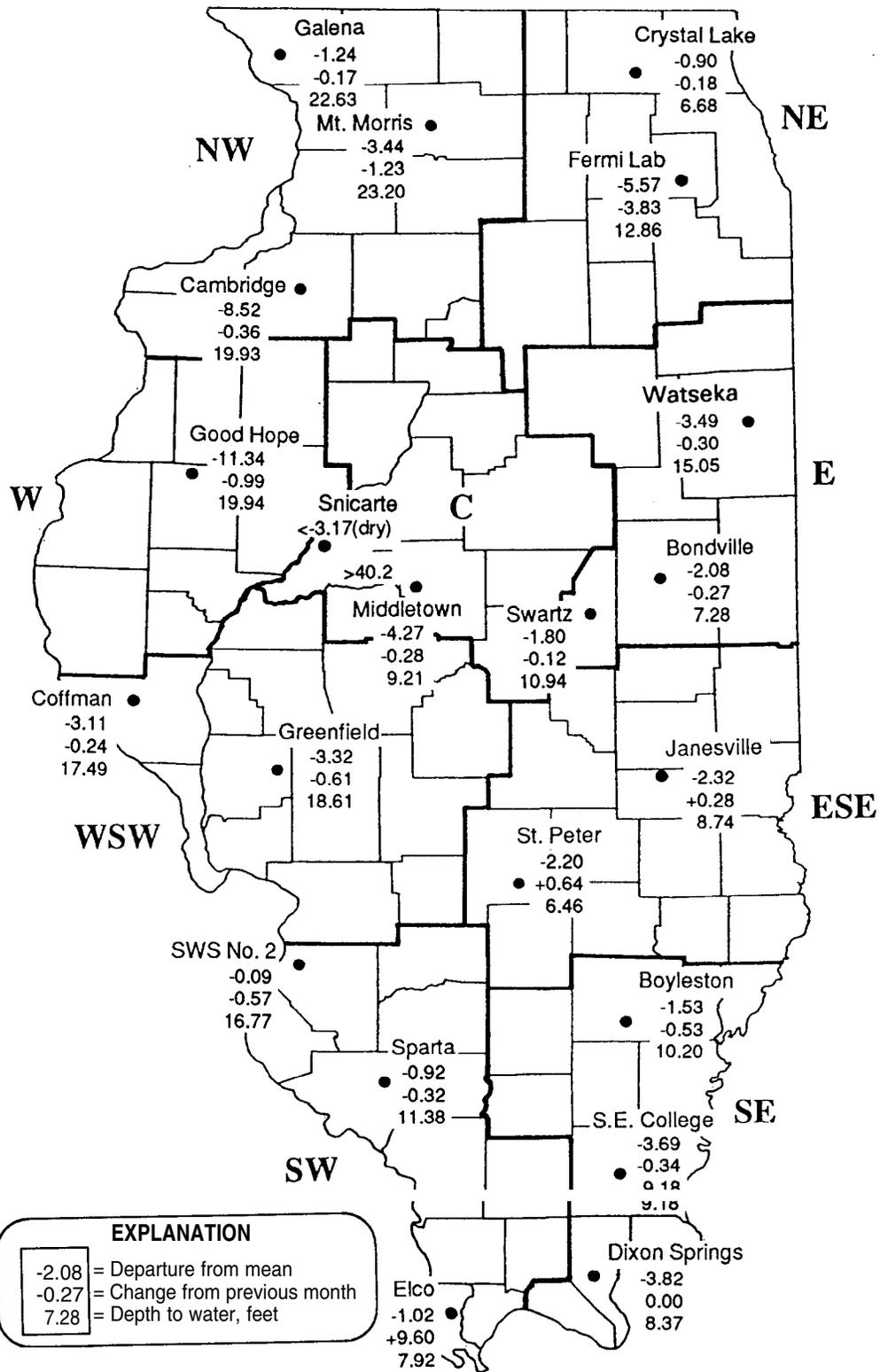
Figure 6.9. Recorded month-end water levels (depth to water), changes from previous month, and departures from mean month-end water levels, October 1988
