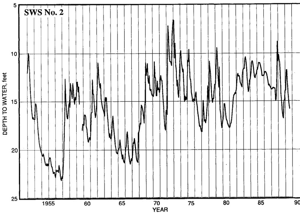
Figure 6.29. Long-term hydrograph for the SWS No. 2 observation well, St. Clair County, 1952-1989. Data are unsmoothed monthly values.
