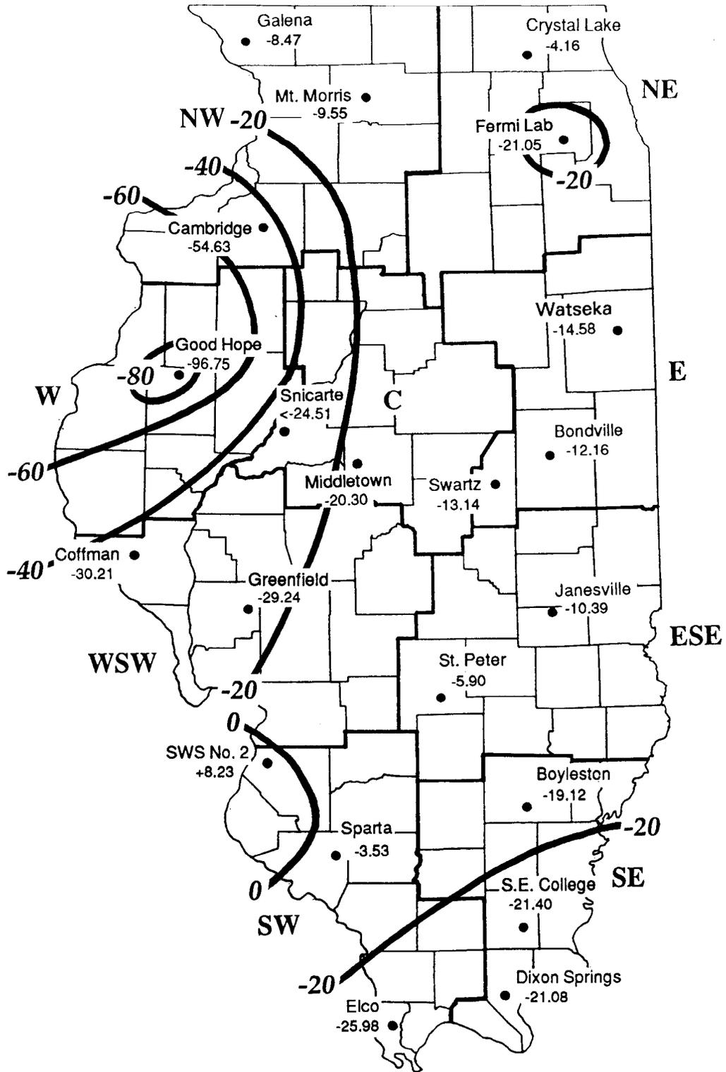
Figure 6.23. Accumulated departures from mean monthly ground-water levels in feet, April - December 1988
