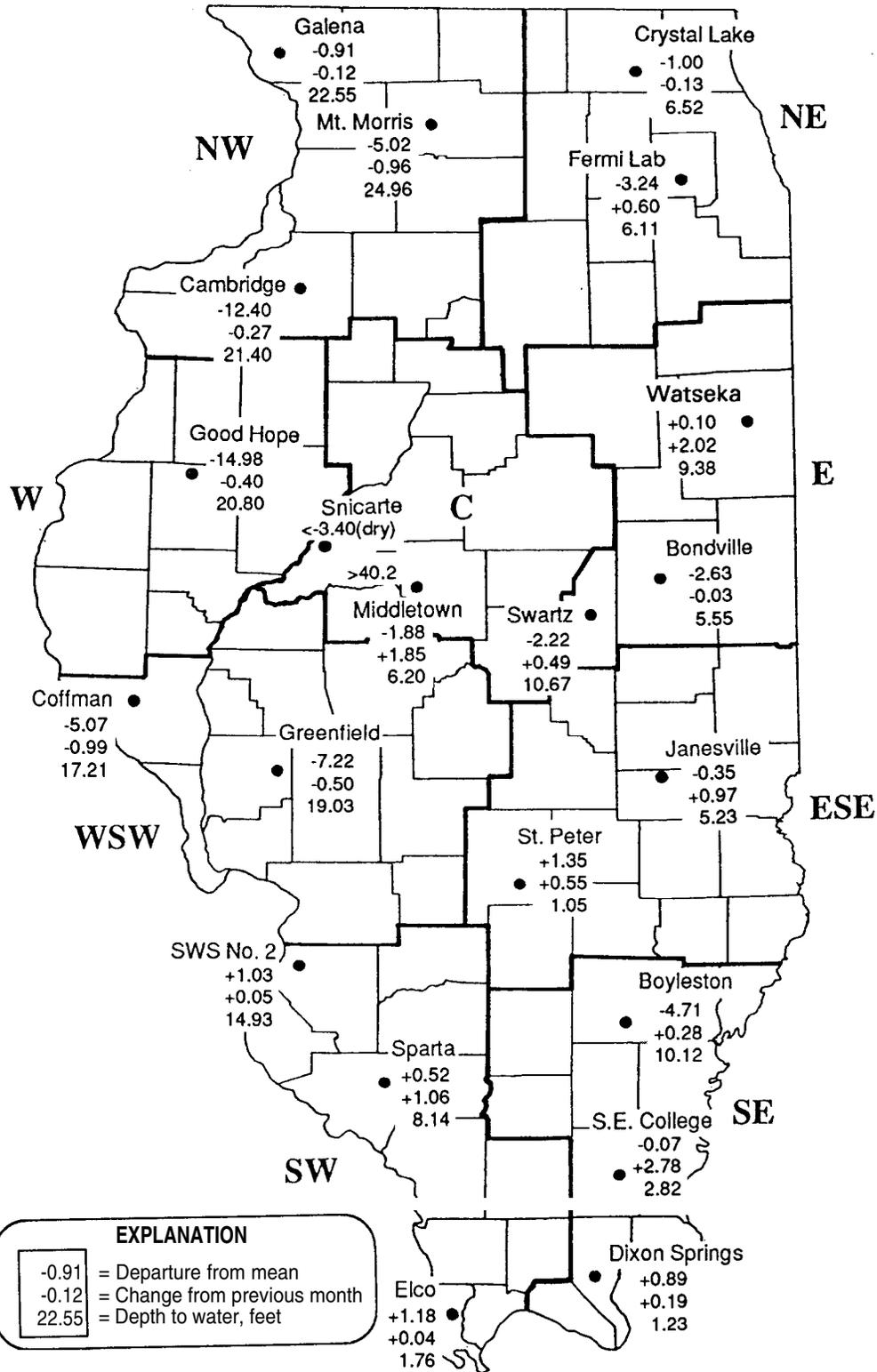
Figure 6.10. Recorded month-end water levels (depth to water), changes from previous month, and departures from mean month-end water levels, December 1988
