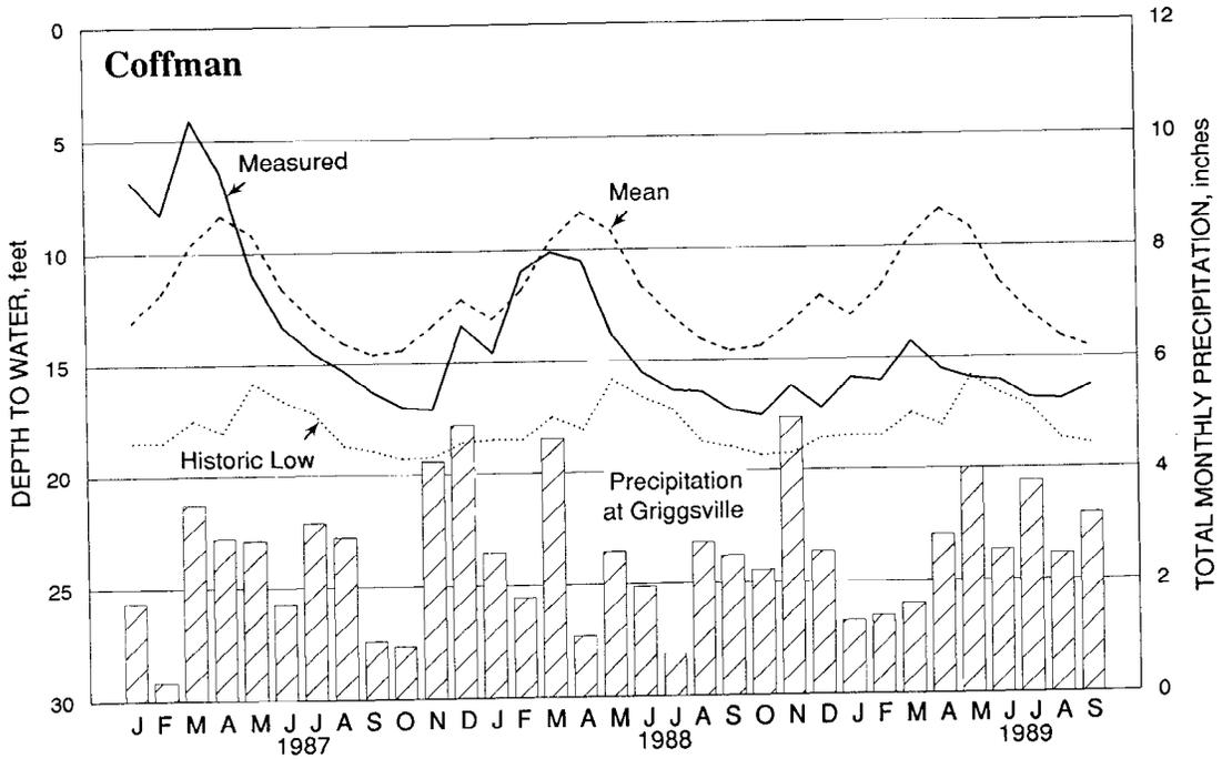
Figure 6.15. Shallow ground-water levels and precipitation at the Coffman observation well, Pike County (west-southwest crop reporting district), January 1987 - September 1989
