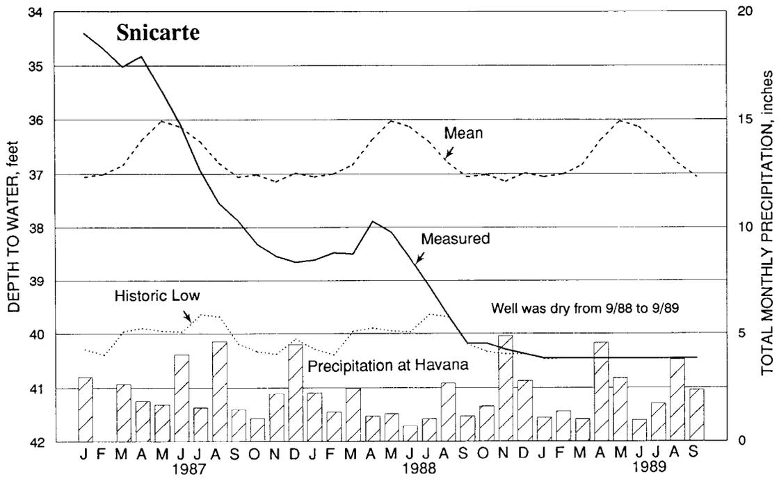
Figure 6.18. Shallow ground-water levels and precipitation at the Snicarte observation well, Mason County (central crop reporting district), January 1987 - September 1989
