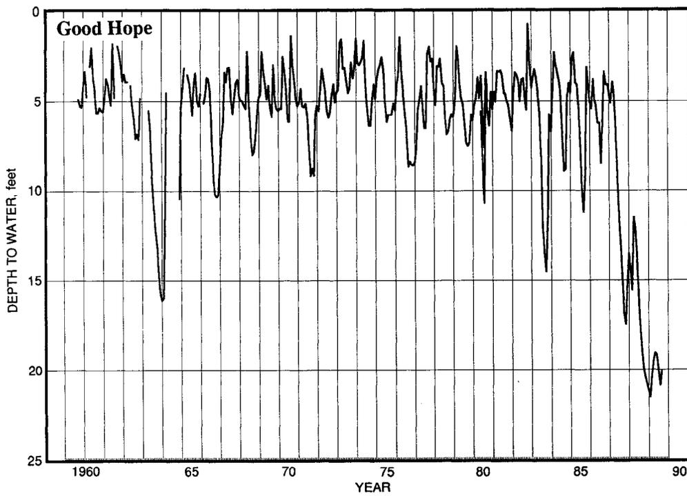
Figure 6.32. Long-term hydrograph for the Good Hope observation well, McDonough County, 1959-1989. Data are unsmoothed monthly values.
