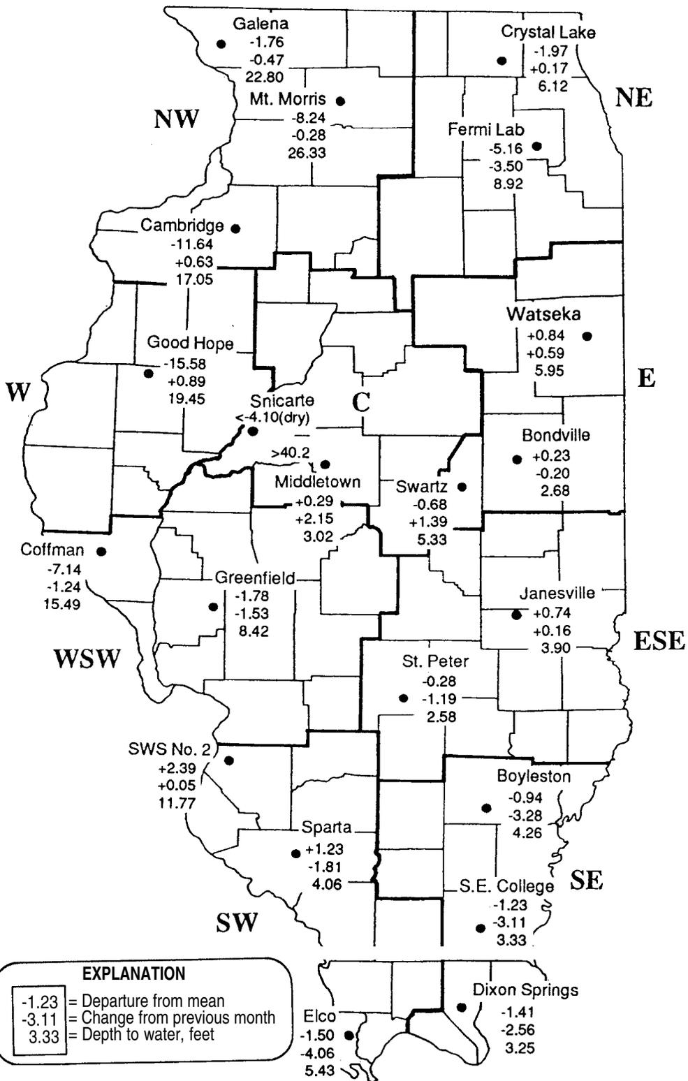
Figure 6.11. Recorded month-end water levels (depth to water), changes from previous month, and departures from mean month-end water levels, April 1989
