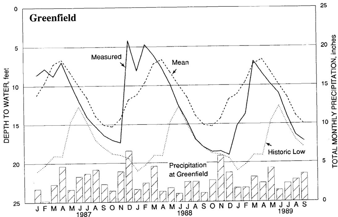
Figure 6.2. Shallow ground-water levels and precipitation at the Greenfield observation well, Greene County (west-southwest crop reporting district), January 1987 - September 1989
