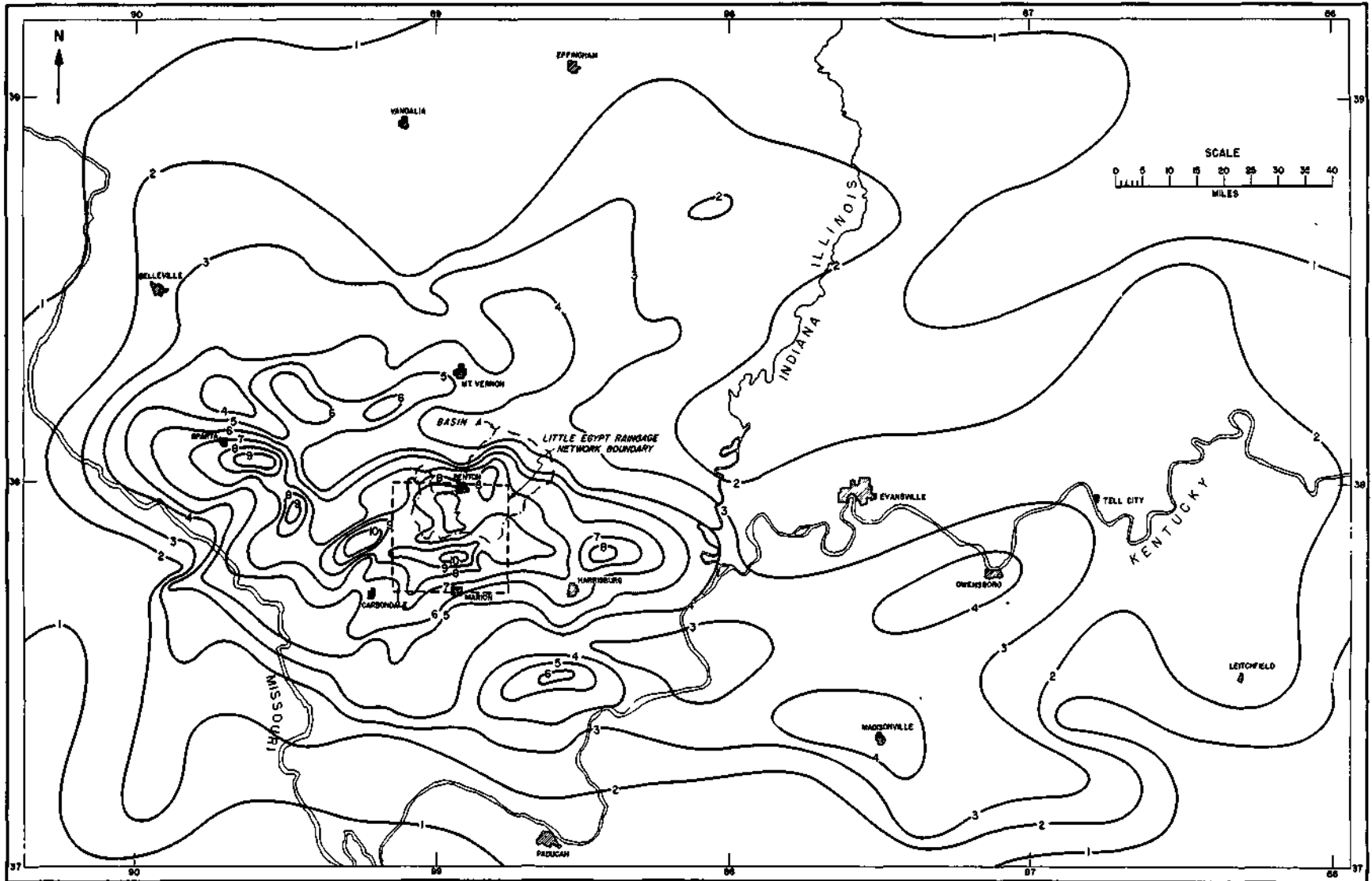
Figure 48. Total storm rainfall for August 16-17, 1959
