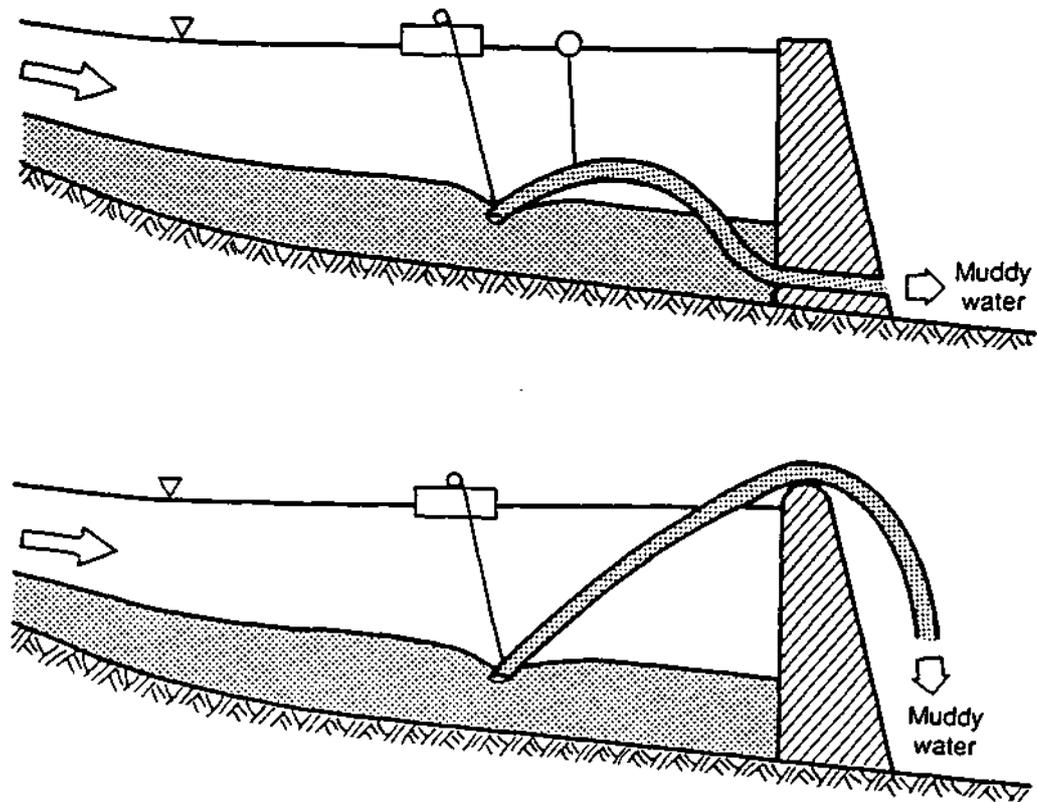
Figure 1. A schematic representation of typical installations of sediment entrapment reduction measures.
