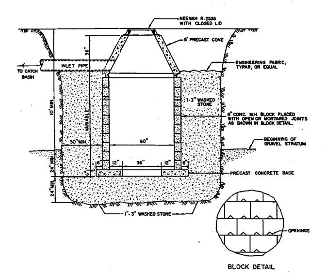
Figure 3. General design of stormwater drainage wells (courtesy of City of Crystal Lake).
