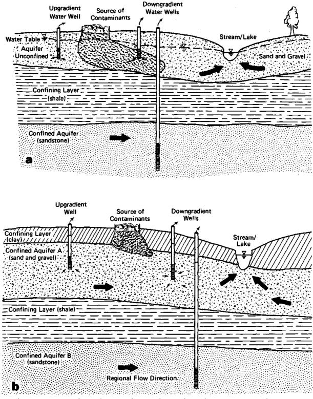
Figure 7. Examples of contaminant plume migration: Case a, plume configuration affected by advection and dispersion only; Case b, plume configuration affected by advection, dispersion, and attenuation in the form of adsorption in the unsaturated clay zone.
