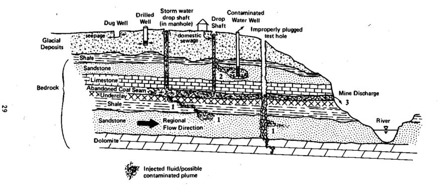
Figure 9. Three possible routes of ground-water contamination after injection of wastes into a coal mine: 1) seepage through cracks or fractures in the underlying shale layer or through an improperly sealed test hole contaminates a deeper aquifer, 2) leakage from an improperly constructed injection/disposal casing allows contaminants to reach an overlying aquifer, or 3) seepage from an exposed face of the coal seam reaches a surface water body.
