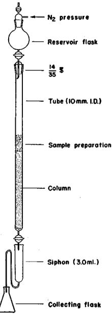
FIGURE 1.—The chromatographic column and related apparatus.
