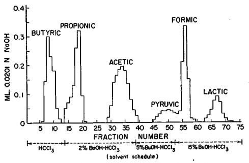
FIGURE 2.—The chromatographic separation of organic acid mixtures.
