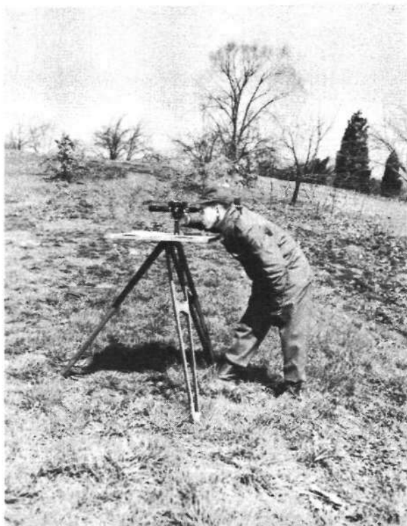
FIG. 21. —PLANETABLE OPERATOR SIGHTING IN POINT OF MEASUREMENT.
