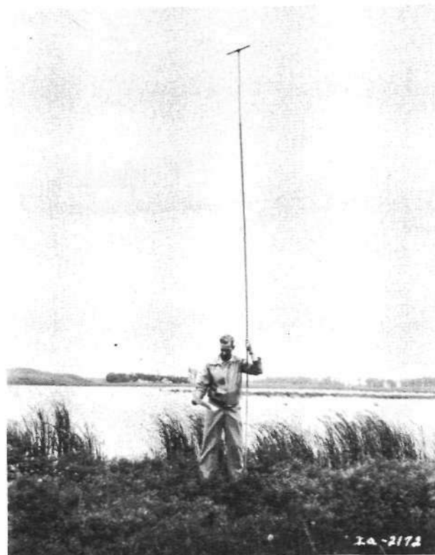
FIG. 22. —EXTENSION AUGER USED FOR SURVEYS OF DRAINED RESERVOIRS.
