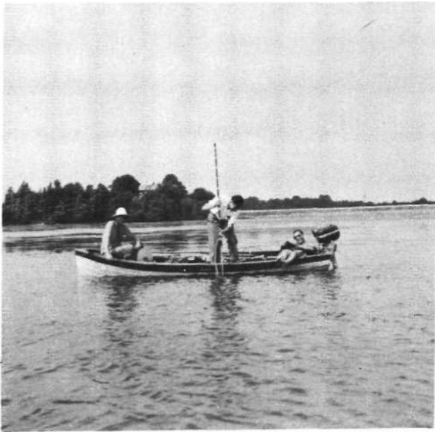
FIG. 23. —USE OF SOUNDING POLE ON LAKE ROCKWELL, OHIO. BOAT IS BEING WINCHED ACROSS LAKE ON "TAG LINE."
