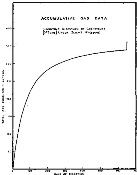
At the end of the experiment the gas cock on the digester was connected to a small gasometer. The weights of the gasometer were regulated so as to produce a slight vacuum (2 inches of water) on the system in order to draw as much of the free and dissolved gases out of the digester as practical. After about four hours the gas collected was measured and analyzed. The digester was then opened, the cornstalks and liquor separated and a complete analysis of each made (Table XLIX).
