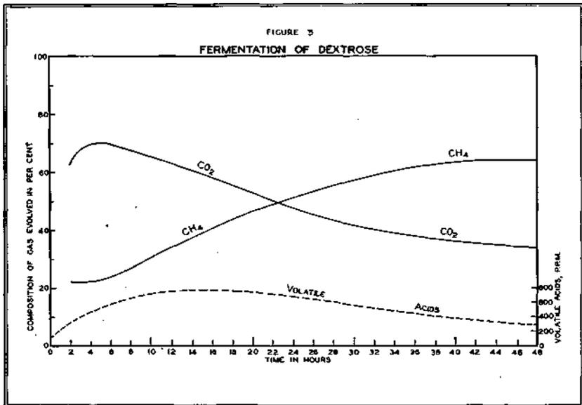
the first six hours of fermentation. Following this, there was a steady downward drift of the carbon dioxide curve and a corresponding upward drift of the methane curve. At thirty-six hours the curves again approached the horizontal and an approximate 3:5 ratio of carbon dioxide to methane continued during the last twelve hours. These ratios would
