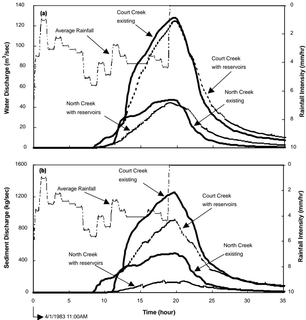
Figure 12. Predicted water and sediment discharges at the North and Court Creek outlets resulting from the April 1, 1983, storm (average rainfall) and assuming two Rice Lake size reservoirs at the two branches of North Creek.
