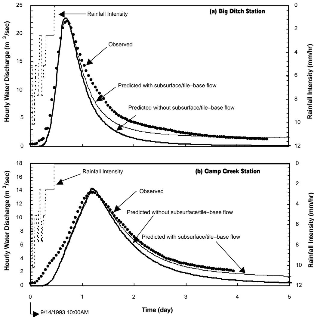
Figure 8. Observed and predicted (with and without subsurface/tile-base flow) hydrographs at (a) Big Ditch and (b) Camp Creek stations resulting from the September 14, 1993, storm.
