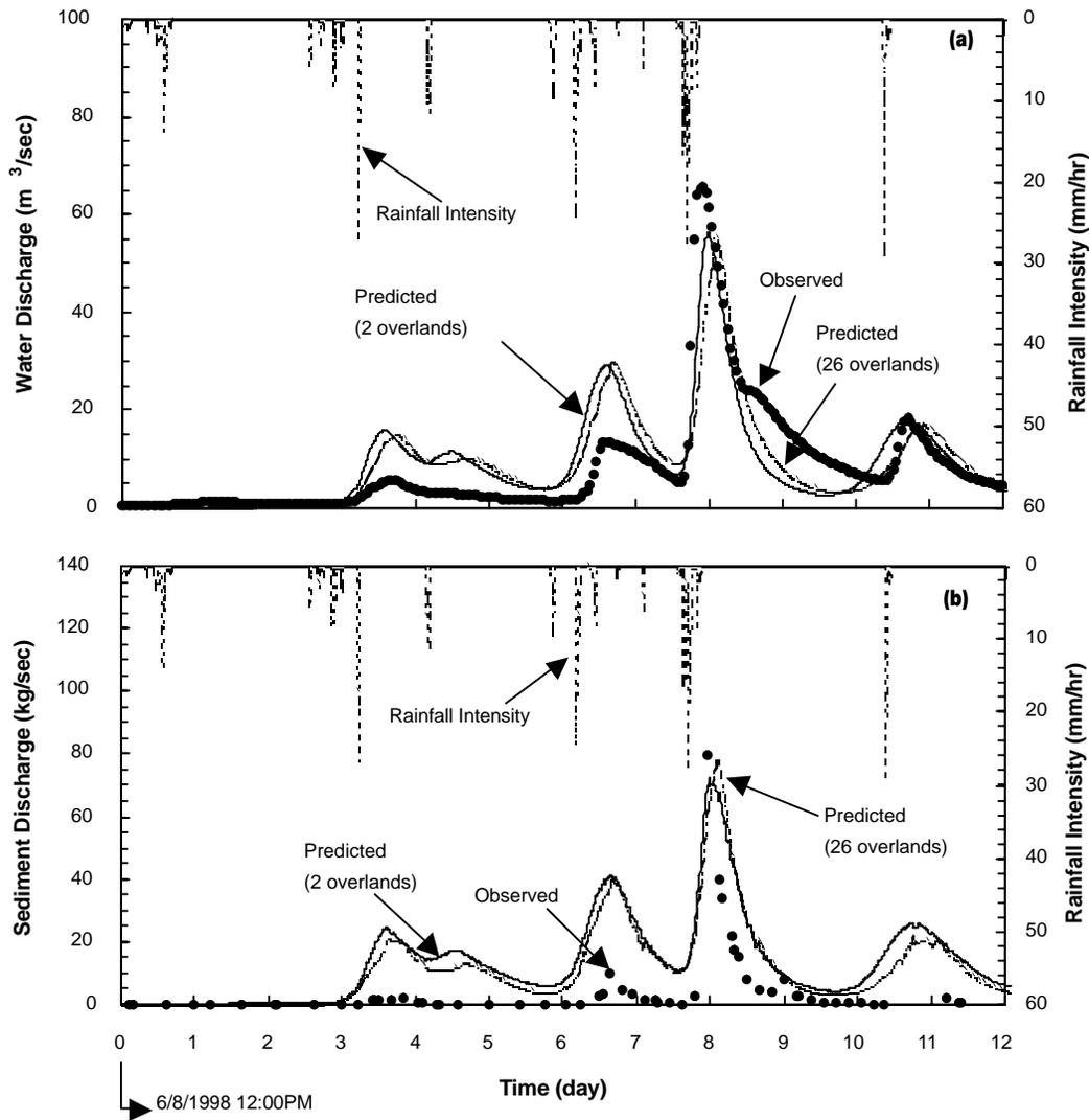
Figure 5. Water and sediment discharges from the Big Ditch watershed divided into coarse (2 overland) and fine (26 overland) subdivisions resulting from the June 1998 storms: Model validation.
