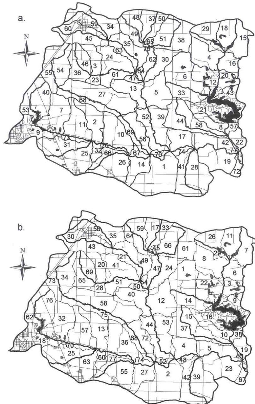
**Figure 10. Ranking of Court Creek watershed overland planes generating highest to the lowest (a) unit-width peak flows and (b) unit-width sediment yields predicted from the April 1, 1983, storm (average rainfall).**
