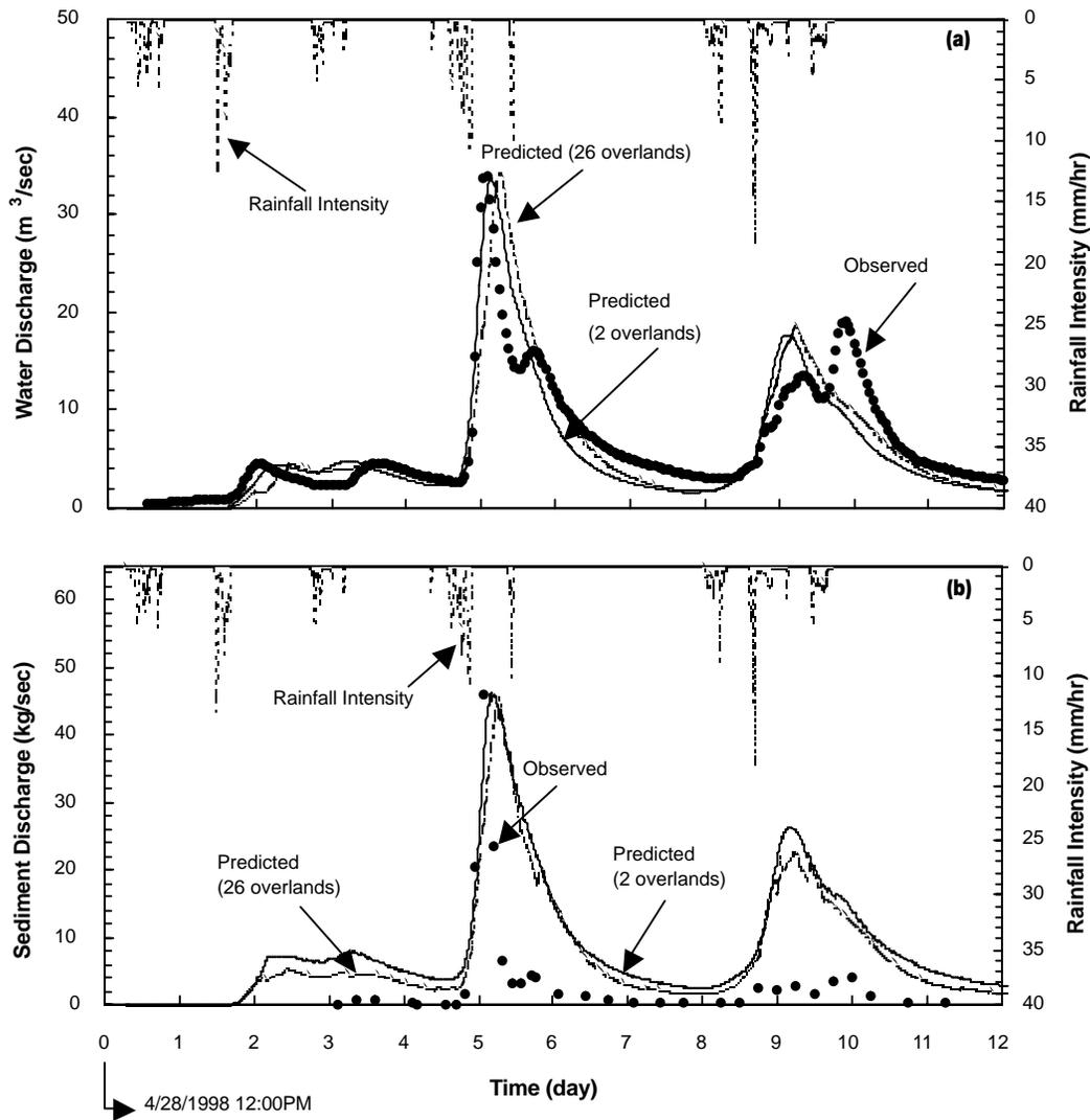
Figure 4. Water and sediment discharges from the Big Ditch watershed divided into coarse (2 overland) and fine (26 overland) subdivisions resulting from the May 1998 storms: Model calibration.
