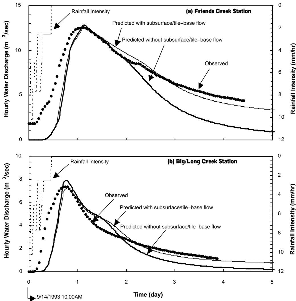
Figure 9. Observed and predicted (with and without subsurface/tile–base flow) hydrographs at (a) Friends Creek and (b) Big/Long Creek stations resulting from the September 14, 1993, storm.
