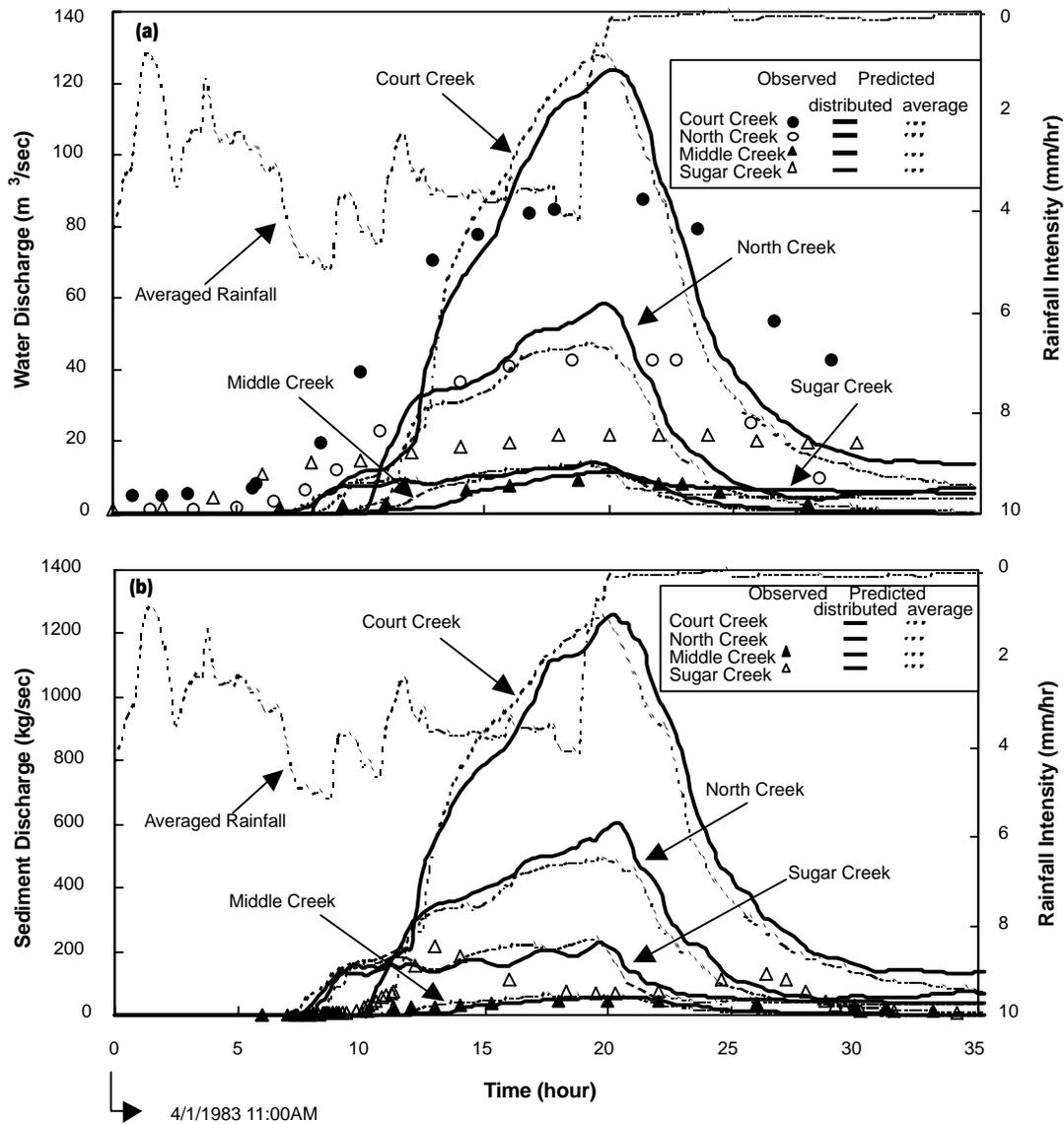
Figure 6. Observed and predicted water and sediment discharges in the Court Creek watershed resulting from spatially distributed and average rainfall of April 1, 1983, storm: Model calibration.
