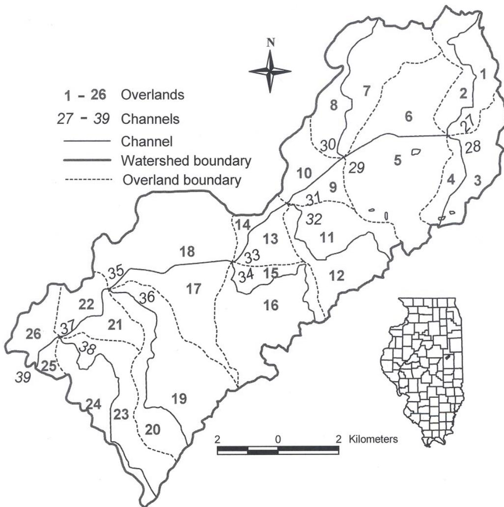
Figure 3. Big Ditch watershed in Illinois divided into 26 overland planes and 13 channel segments.
