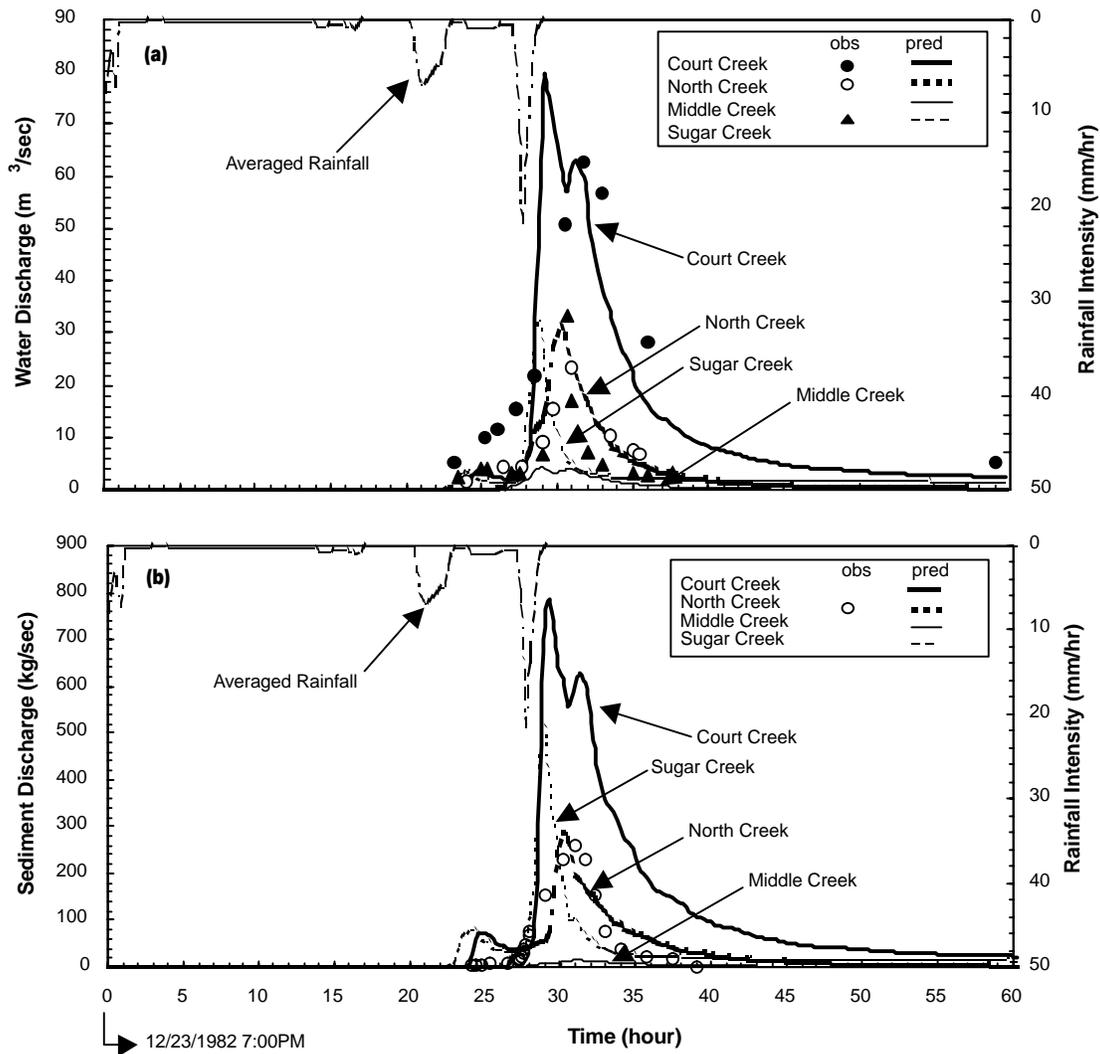
Figure 7. Observed and predicted water and sediment discharges in the Court Creek watershed resulting from the December 24, 1982, storm (distributed rainfall): Model validation.
