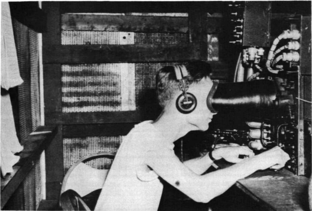
Fig. 1. Radar operator studying the PPI scope. Earphone indicate readiness to communicate with the aircraft.
