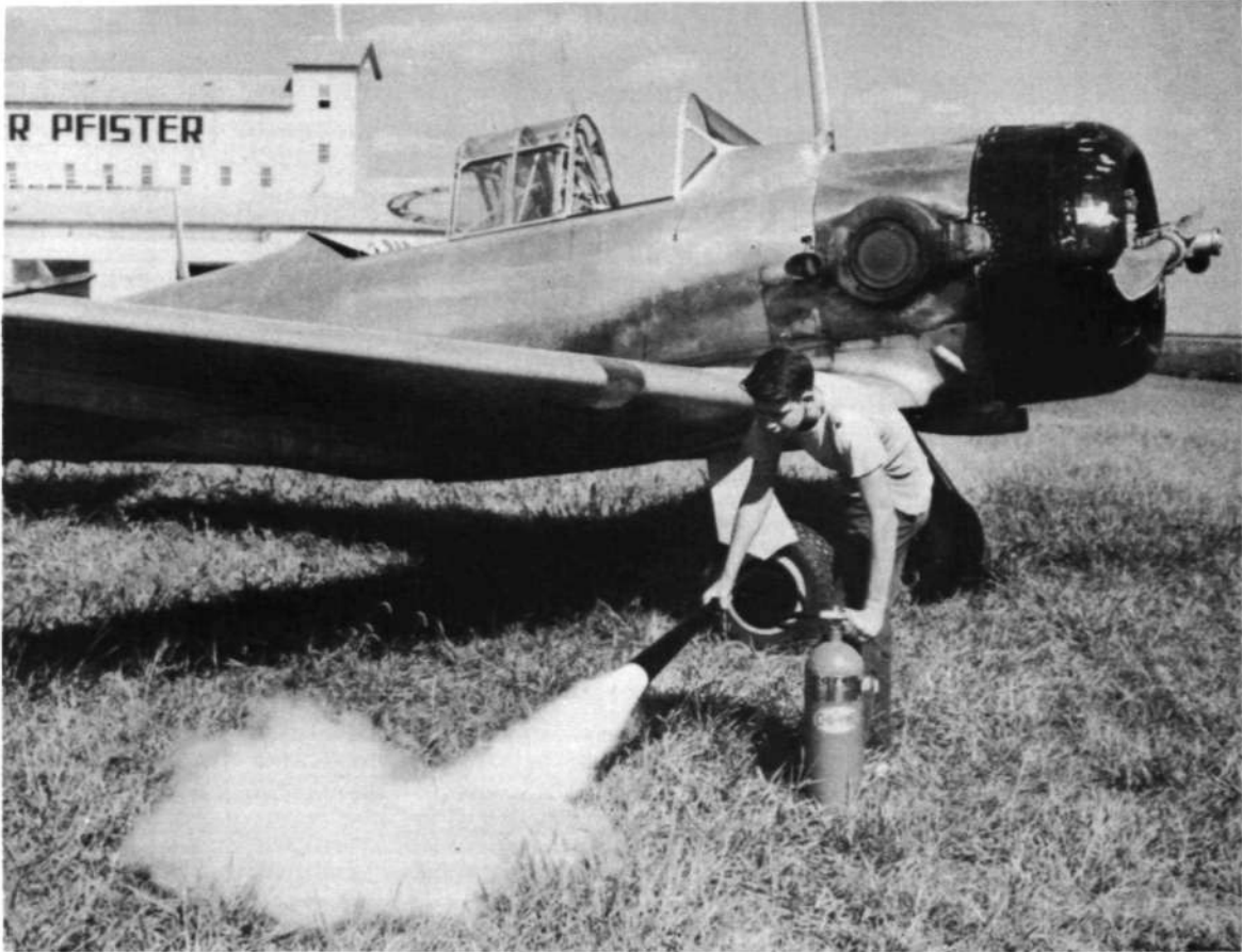
Fig. 5. AT-6 Aircraft with super-charger. CO 2 extinguisher producing small particles of dry ice.
