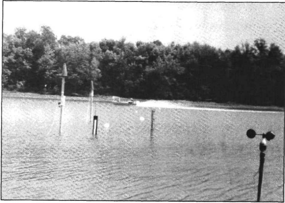
Figure 8. Instrumentation setup at the Havana site (Note wind set 2, installed at a height of 1 meter at the water and bankline interface)
