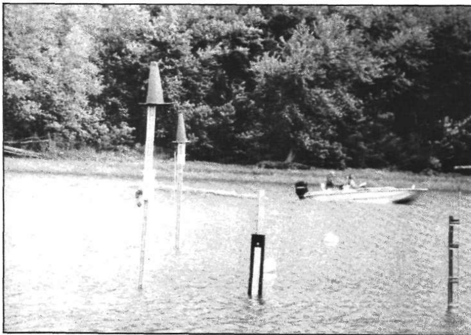
Figure 9. Wave gages and staff gage setup at the Havana site
