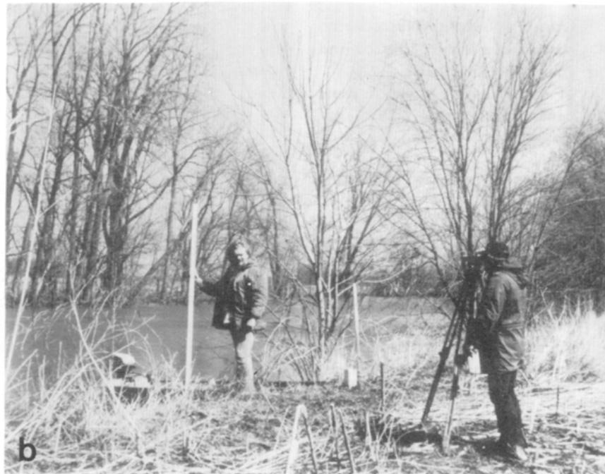
Figure 9. Water surface elevation determination
