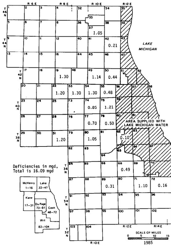
Figure 29. Water demands in 1985 in excess of groundwater available from natural recharge and mining limited to 1980 pumpage (scheme 3)
