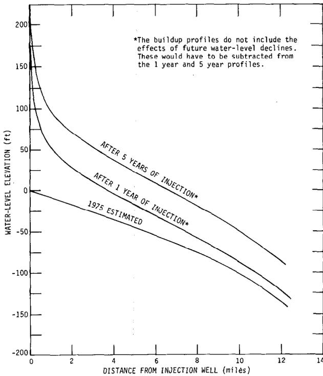
Figure 53. Piezometric profiles, Central Park Avenue pumping station
