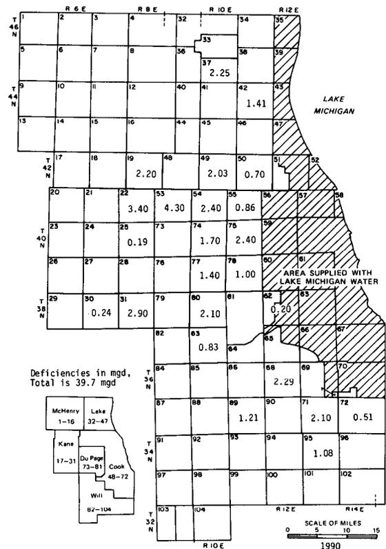
Figure 30. Water demands in 1990 in excess of groundwater available from natural recharge and mining limited to 1980 pumpage (scheme 3)
