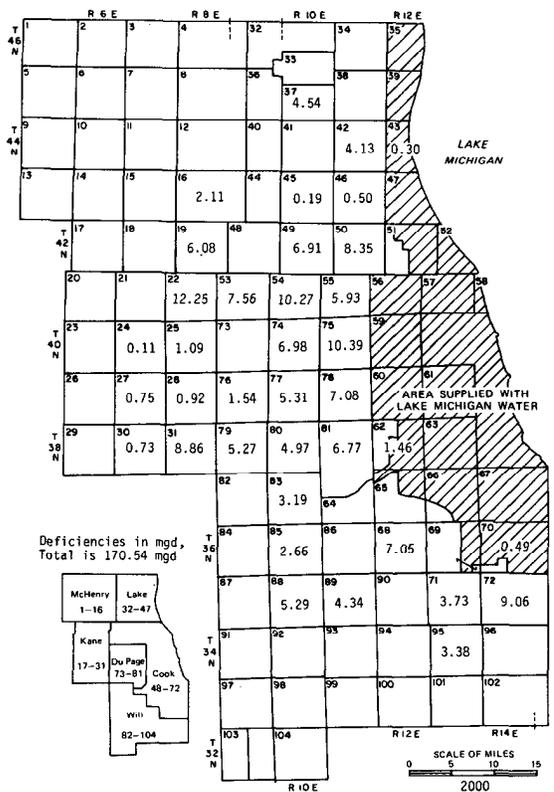
Figure 19. Water demands in 2000 in excess of groundwater available from natural recharge
