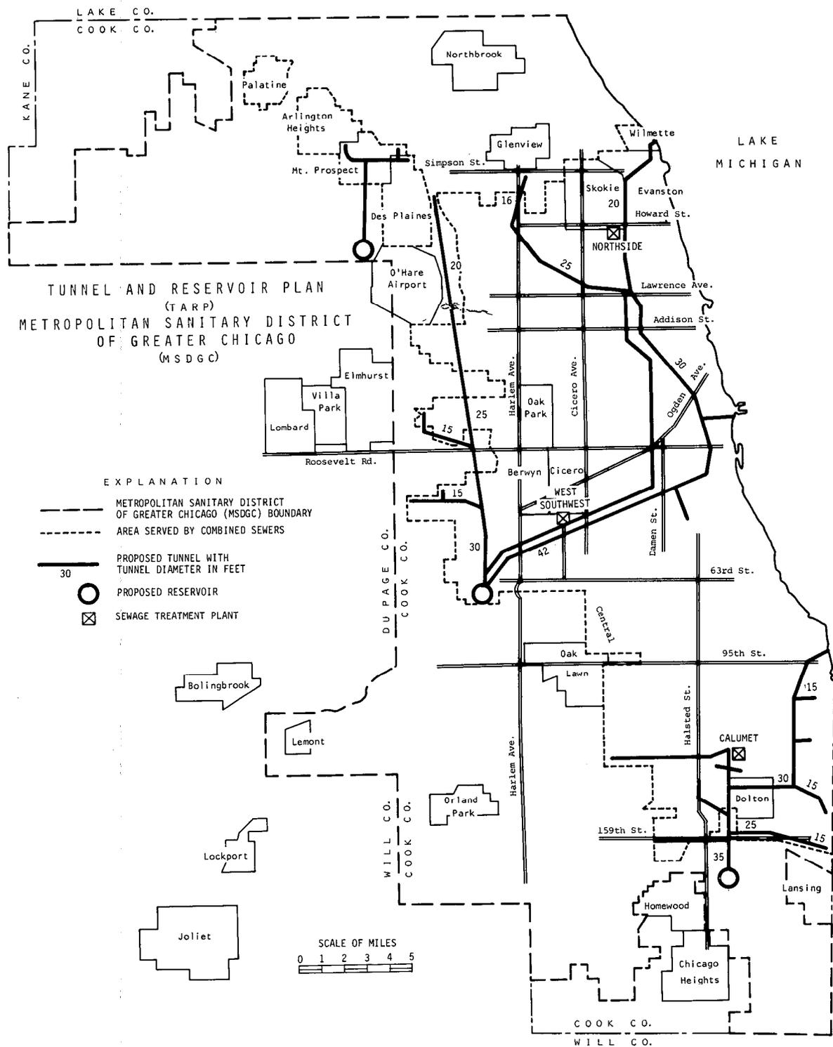
Figure 59. Layout of Chicago Tunnel and Reservoir Plan (TARP)
