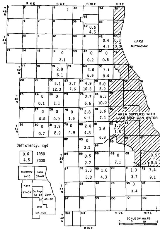
Figure 37. Water demands in excess of groundwater available from natural recharge
