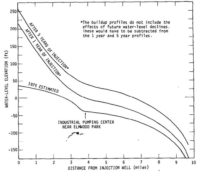
Figure 52. Piezometric profiles, Springfield Avenue pumping station
