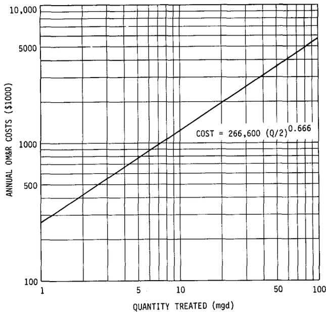
Figure 35. Annual operation, maintenance, and repair costs of treatment plants versus quantity treated
