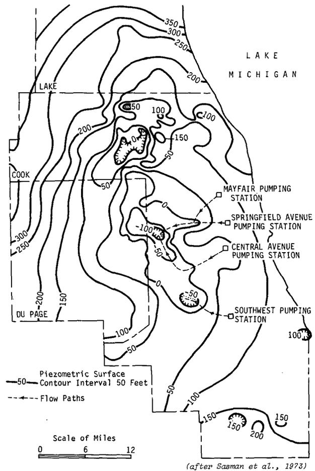
Figure 49. Elevation of piezometric surface of Cambrian-Ordovician aquifer (deep sandstone), October 1971
