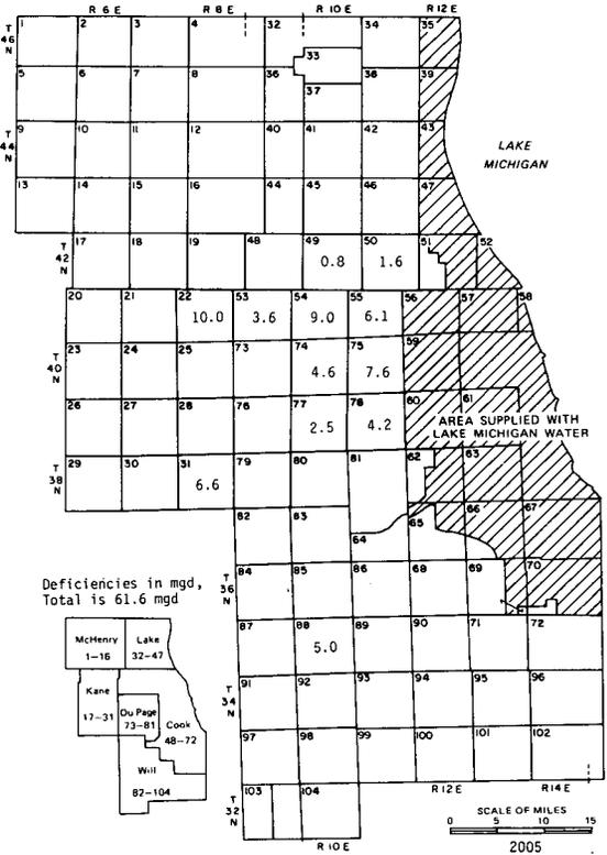
Figure 23. Water demands in 2005 in excess of groundwater available from natural recharge and mining (scheme 1)
