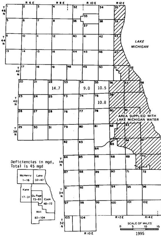
Figure 25. Water demands in 1995 in excess of groundwater available from natural recharge and mining (scheme 2)
