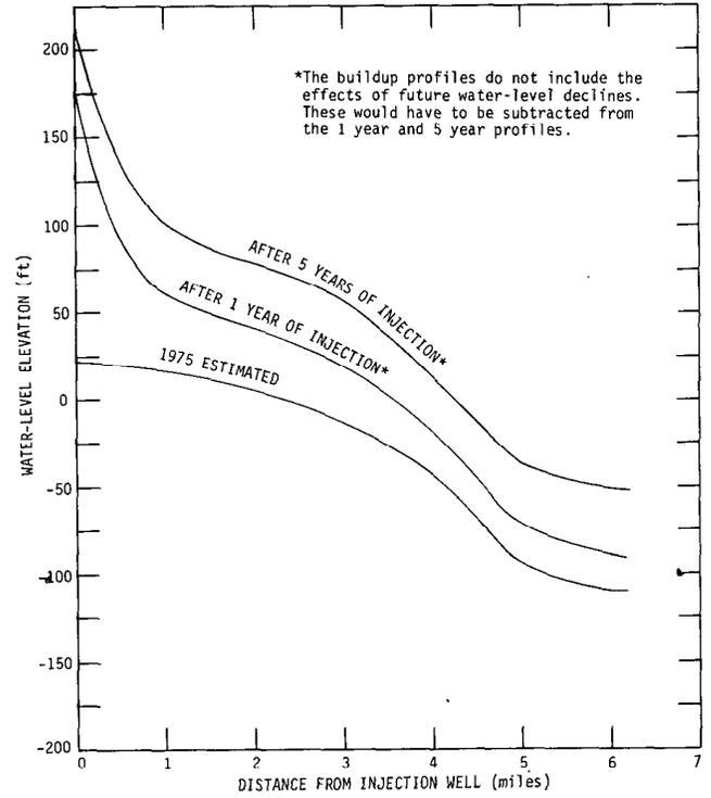
Figure 54. Piezometric profiles, Southwest pumping station
