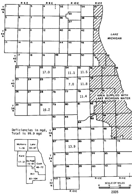
Figure 27. Water demands in 2005 in excess of groundwater available from natural recharge and mining (scheme 2)
