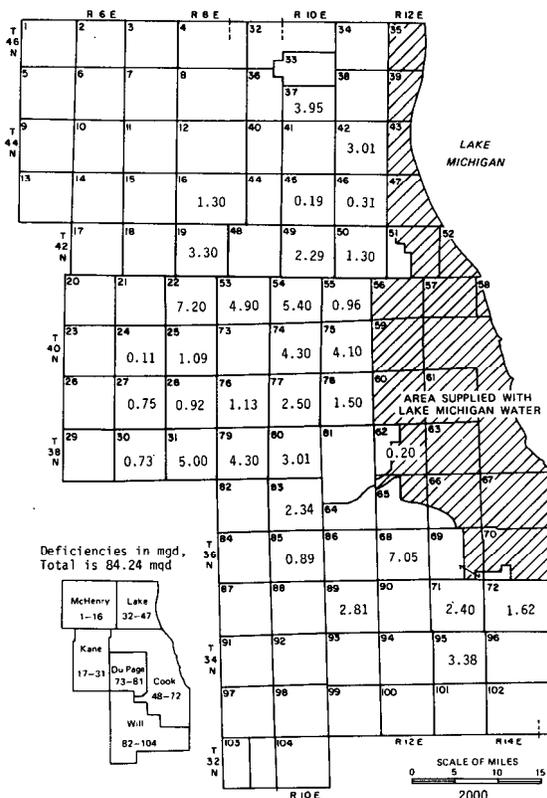
Figure 31. Water demands in 2000 in excess of groundwater available from natural recharge and mining limited to 1980 pumpage (scheme 3)
