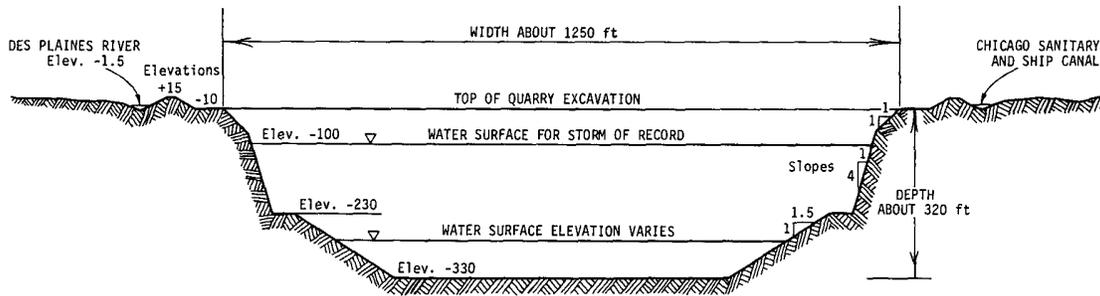
Figure 62. Cross section of proposed surface reservoir near McCook
