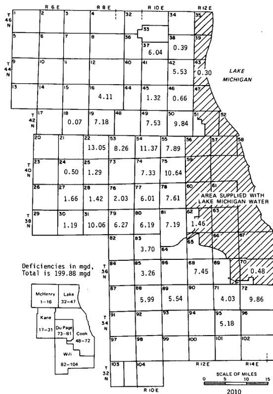
Figure 20. Water demands in 2010 in excess of groundwater available from natural recharge
