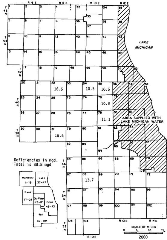
Figure 26. Water demands in 2000 in excess of groundwater available from natural recharge and mining (scheme 2)
