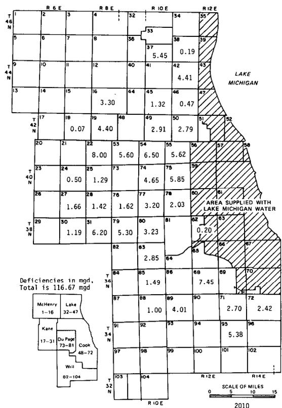
Figure 32. Water demands in 2010 in excess of groundwater available from natural recharge and mining limited to 1980 pumpage (scheme 3)
