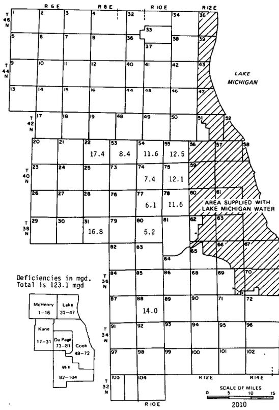
Figure 28. Water demands in 2010 in excess of groundwater available from natural recharge and mining (scheme 2)
