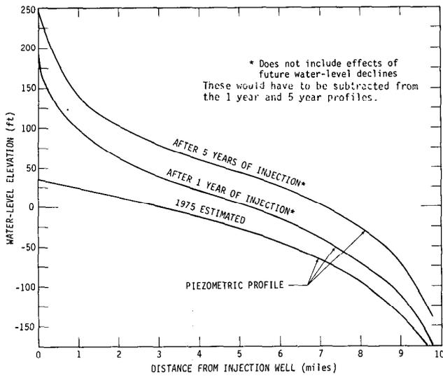
Figure 51. Piezometric profiles, Mayfair pumping station
