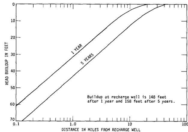
Figure 50. Piezometric head buildup in the deep sandstone aquifer for 1000 gpm recharge rate
