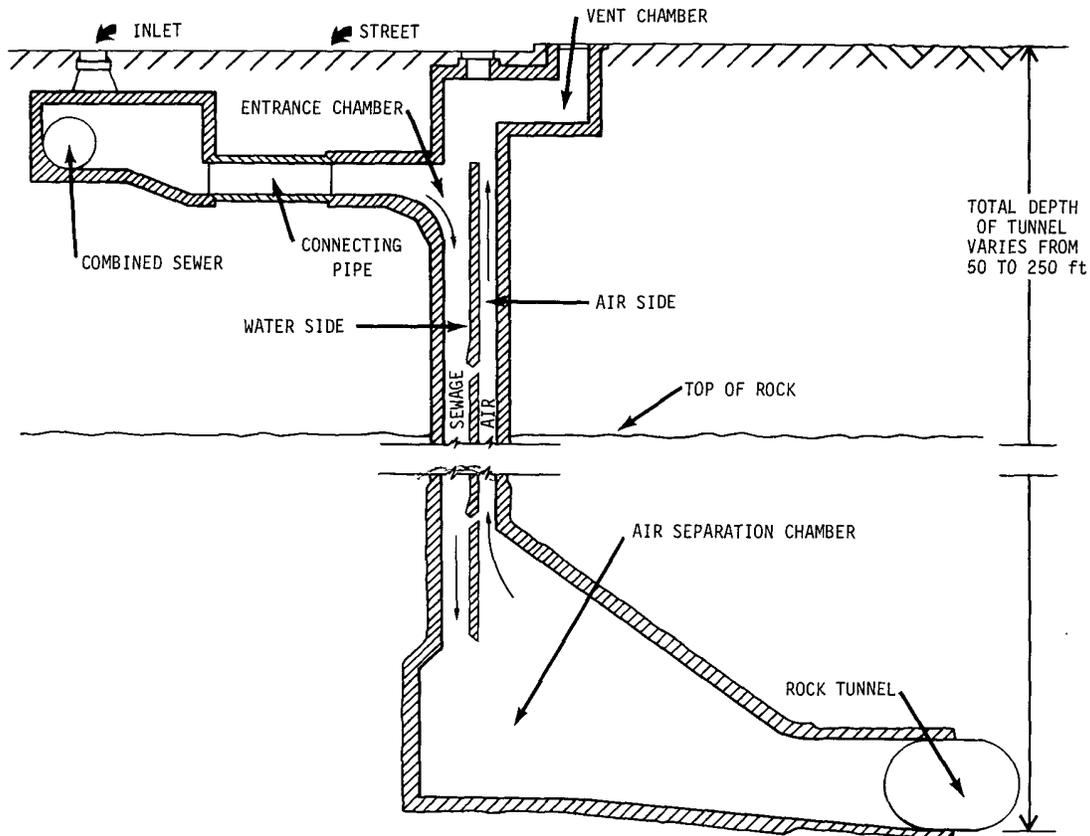
Figure 60. Cross section of vertical drop shaft
