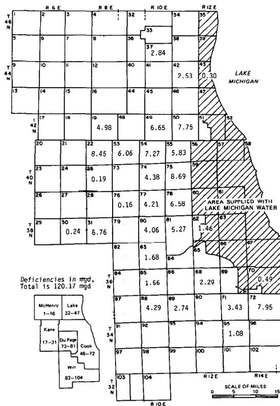
Figure 18. Water demands in 1990 in excess of groundwater available from natural recharge
