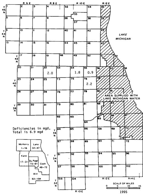
Figure 21. Water demands in 1995 in excess of groundwater available from natural recharge and mining (scheme 1)
