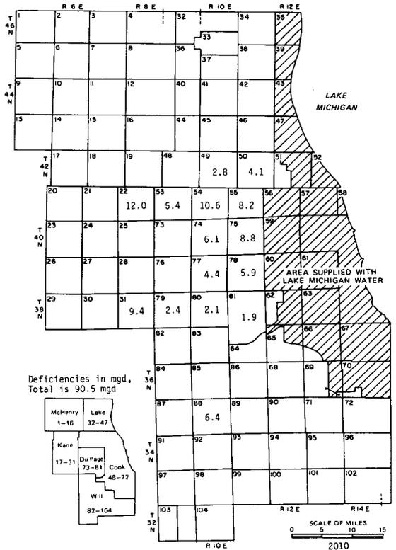
Figure 24. Water demands in 2010 in excess of groundwater available from natural recharge and mining (scheme 1)
