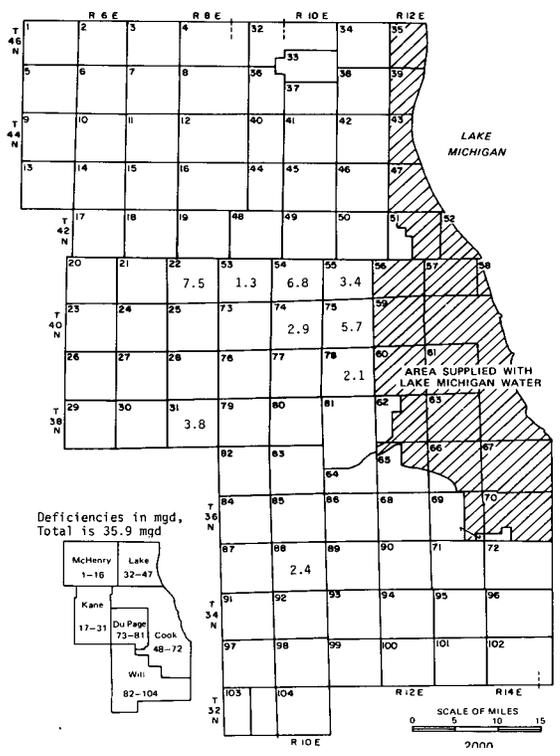
Figure 22. Water demands in 2000 in excess of groundwater available from natural recharge and mining (scheme 1)
