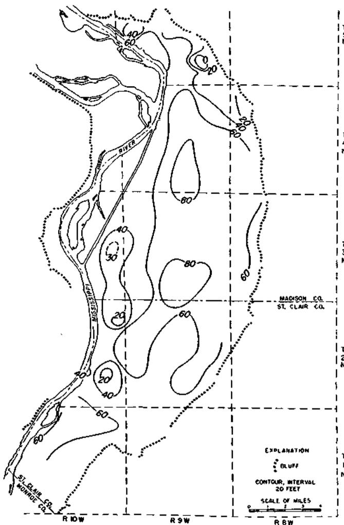
Figure 65. Estimated available drawdown to top of medium sand and coarser deposits in June 1962
