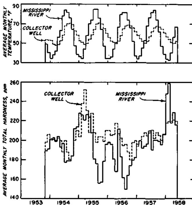
Figure 71. Chemical and temperature data for collector well and Mississippi River, 1953-1958
