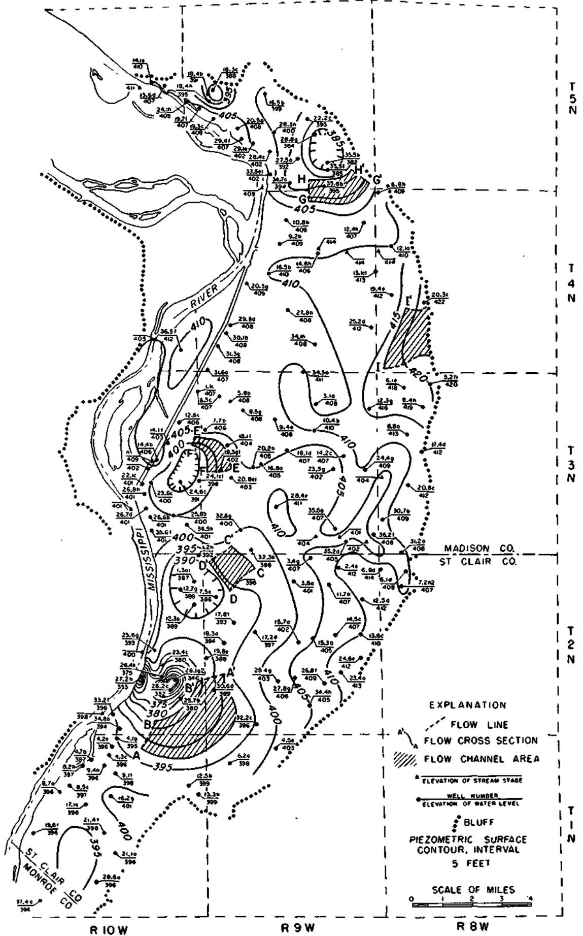
Figure 54. Approximate elevation of piezometric surface, June 1962
