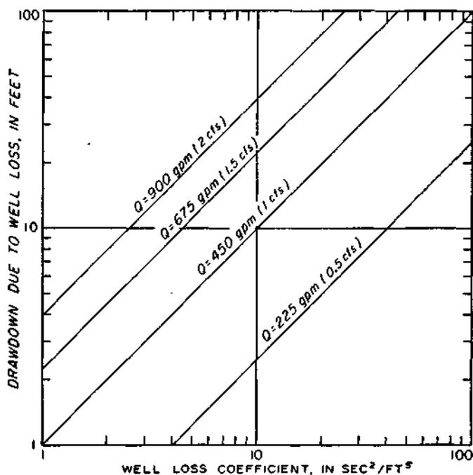
Figure 29. Relation between well-loss constant and drawdown due to well loss
