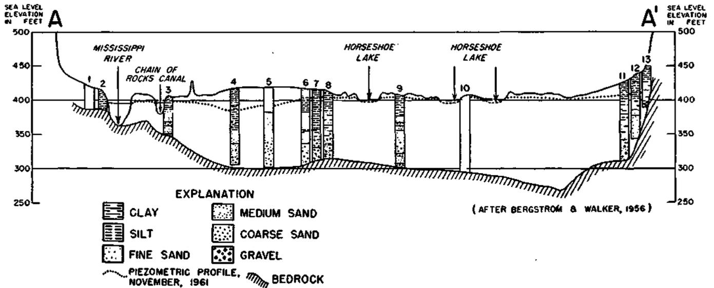
Figure 7. Geologic cross section and piezometric profile of the valley fill
