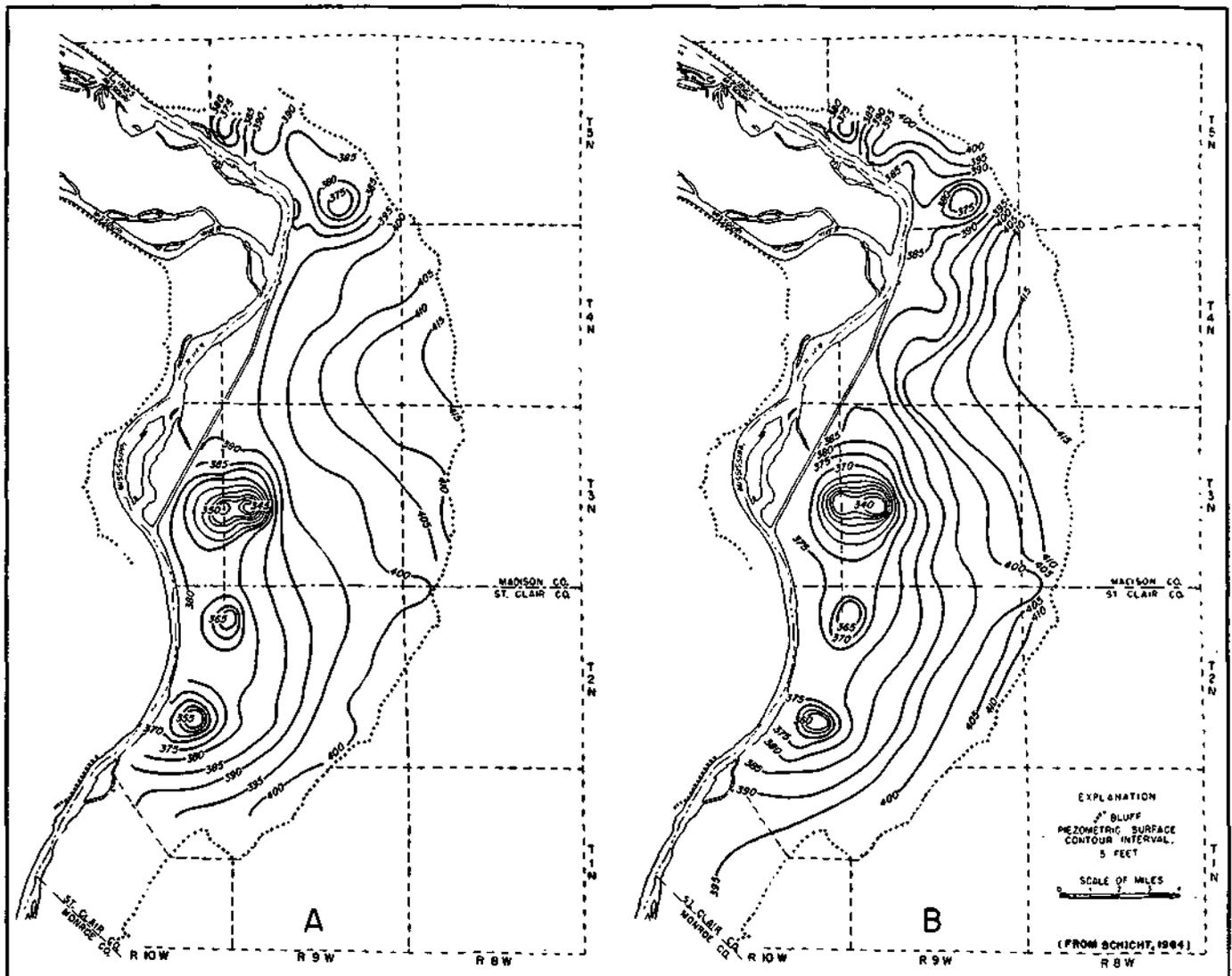
Figure 61. Elevation of piezometric surface, December 1956, actual (A), based on analog computer results (B)
