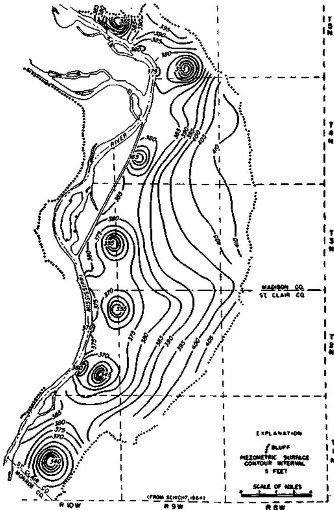
Figure 68. Approximate elevation of piezometric surface with a selected scheme of development
