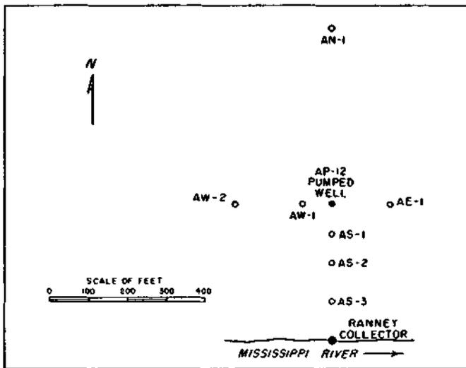
Figure 17. Location of wells used in aquifer test 5
