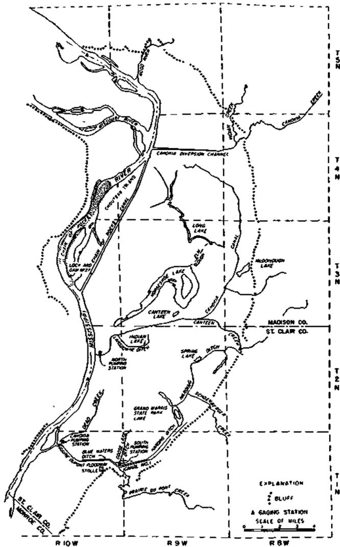
Figure 2. Drainage system and locations of stream-gaging stations
