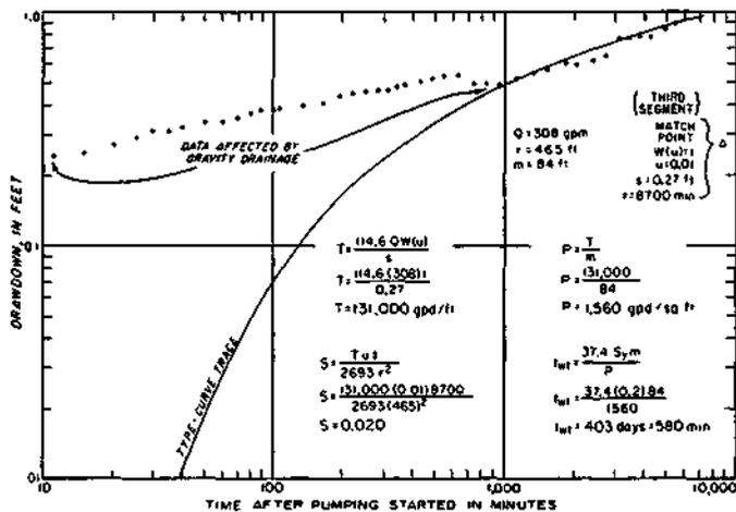
Figure 12. Time-drawdown data for observation well 2, aquifer test 2
