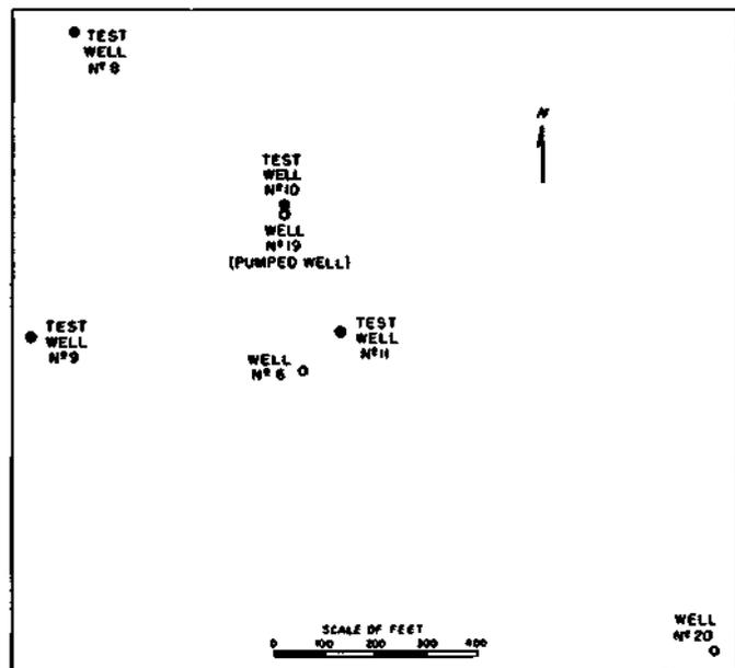
Figure 9. Location of wells used in aquifer test 1
