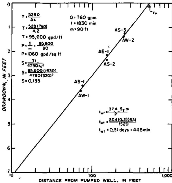
Figure 18. Distance-drawdown data for aquifer test 5
