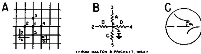
Figure 60. Finite-difference grid (A), resistor-capacitor net (B), and pumping rate oscilloscope trace (C)
