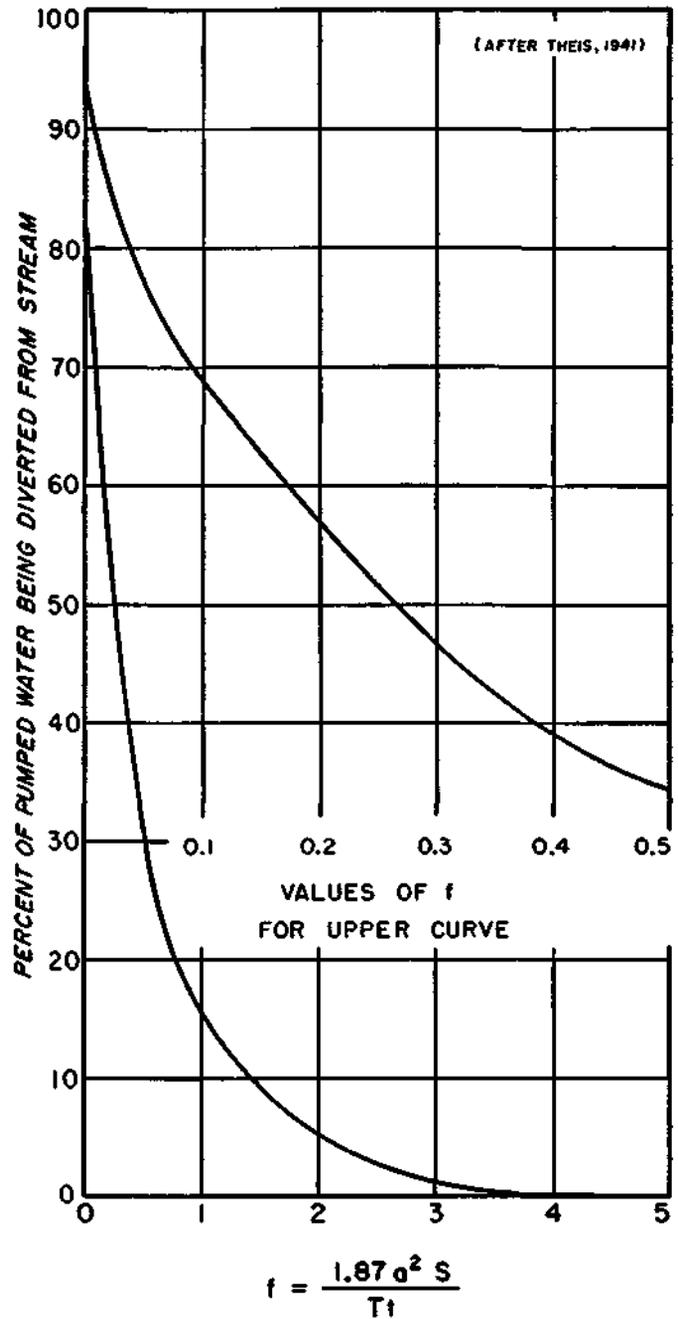
Figure 55. Graph showing the relationship between percent of pumped water being diverted from a stream and the factor 'f'
