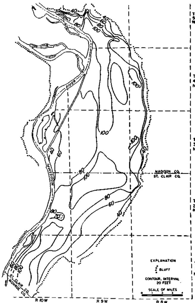
Figure 24. Saturated thickness of aquifer, November 1961
