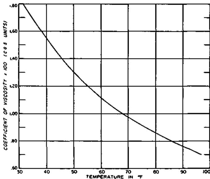
**Figure 56. Graph showing relationship between coefficient of viscosity and temperature**
