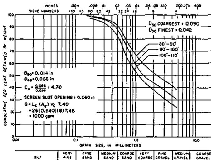
Figure 31. Mechanical analyses of samples for test hole
