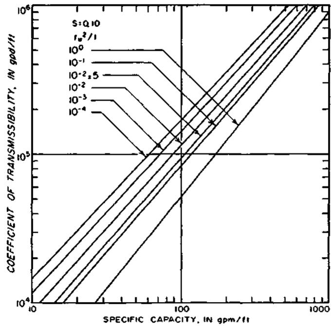
Figure 22. Coefficient of transmissibility versus specific capacity for several values of well radius and pumping period
