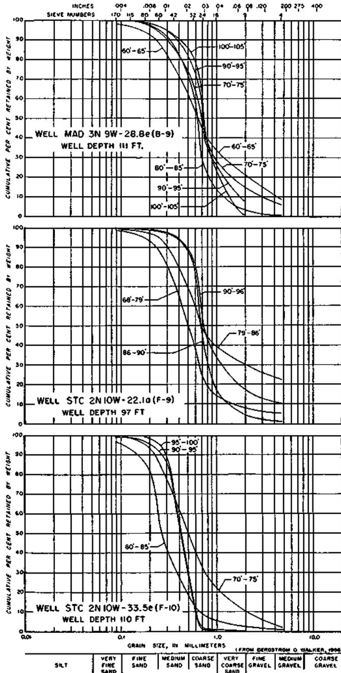
Figure 28. Mechanical analyses of samples from wells
