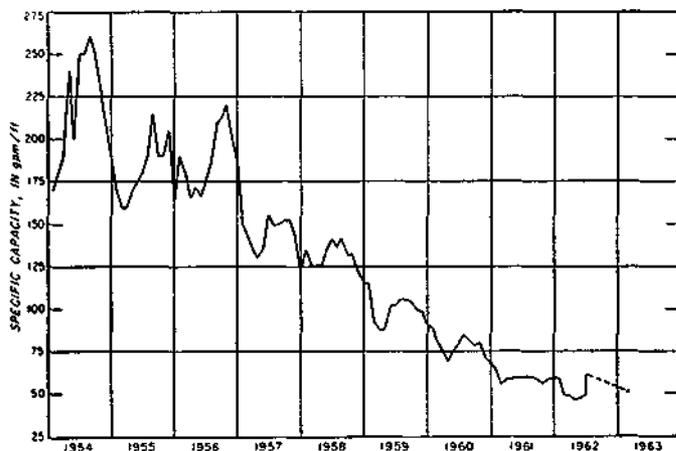
Figure 30. Specific-capacity data for collector well, 1954 to March 1963
