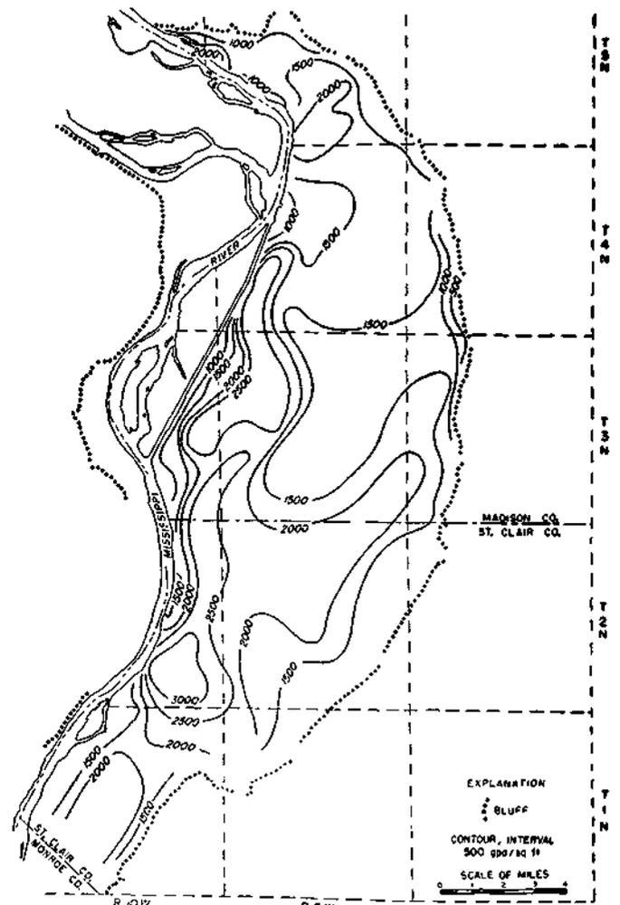
Figure 23. Coefficient of permeability of aquifer
