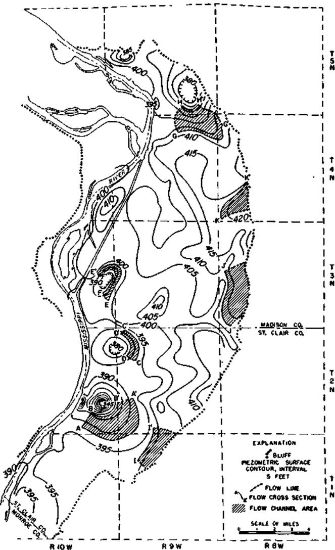
Figure 53. Approximate elevation of piezometric surface, June 1961
