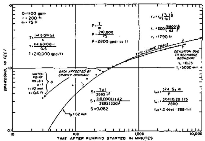
Figure 20. Time-drawdown data for well S-2, aquifer test 6
