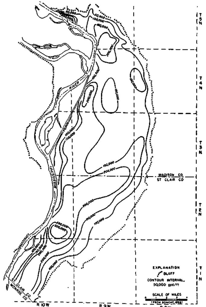
Figure 25. Coefficient of transmissibility of aquifer
