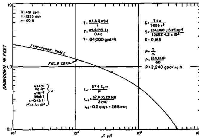
Figure 14. Distance-drawdown data for aquifer test 3
