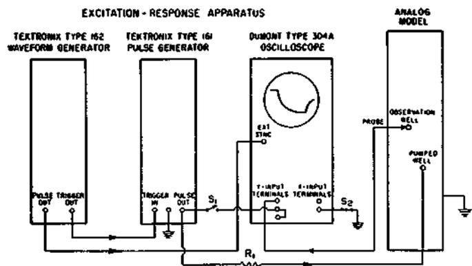
Figure 59. Schematic diagram of electric analog computer
