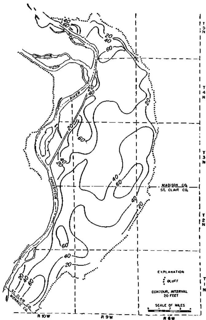
Figure 64. Thickness of medium sand and coarser deposits in lower part of valley fill
