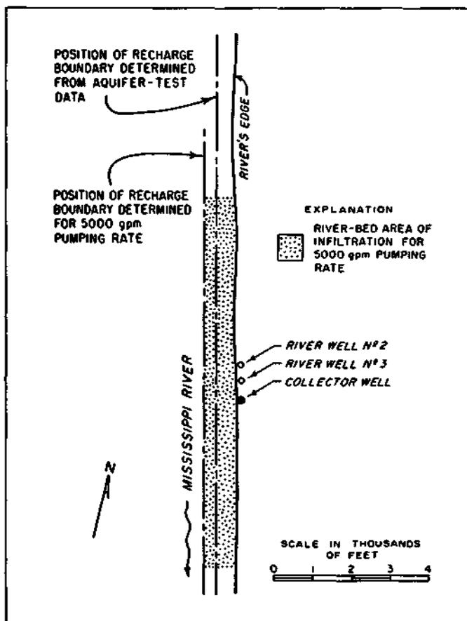
Figure 58. River-bed area of infiltration for Shell Oil Refinery well field
