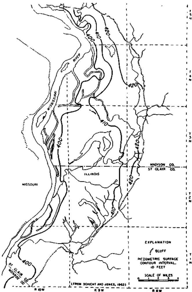
Figure 51. Drainage system and estimated elevation of piezometric surface about 1900
