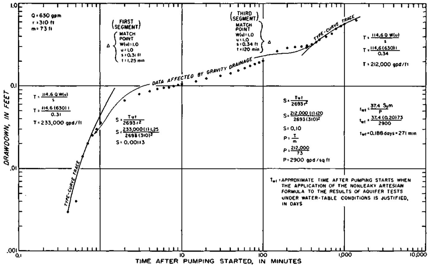
Figure 10. Time-drawdown data for well 6, aquifer test 1
