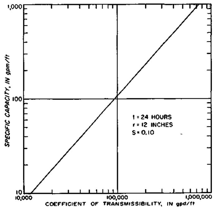
Figure 21. Theoretical relation between specific capacity and the coefficient of transmissibility
