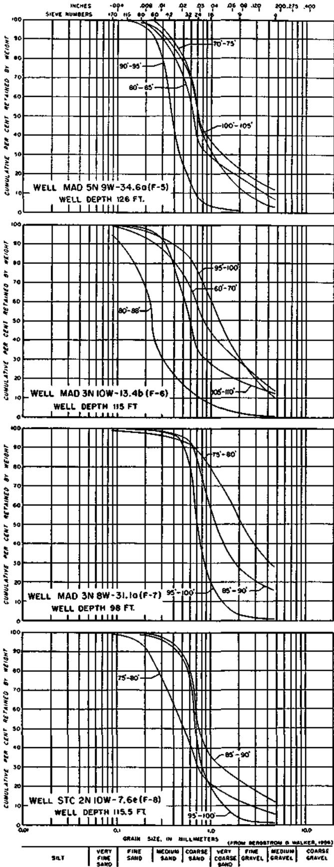
Figure 27. Mechanical analyses of samples from wells
