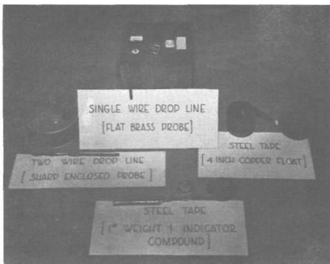
FIG. 28 - COMMON FIELD METHOD OF WATER LEVEL MEASUREMENTS THAT WERE TESTED IN THE LABORATORY WELL.
