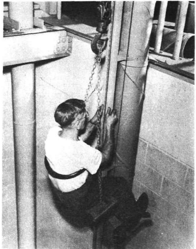
FIG. 21-TAKING READINGS ON LEG 2 OF THE LABORATORY WELL PIEZOMETER.
