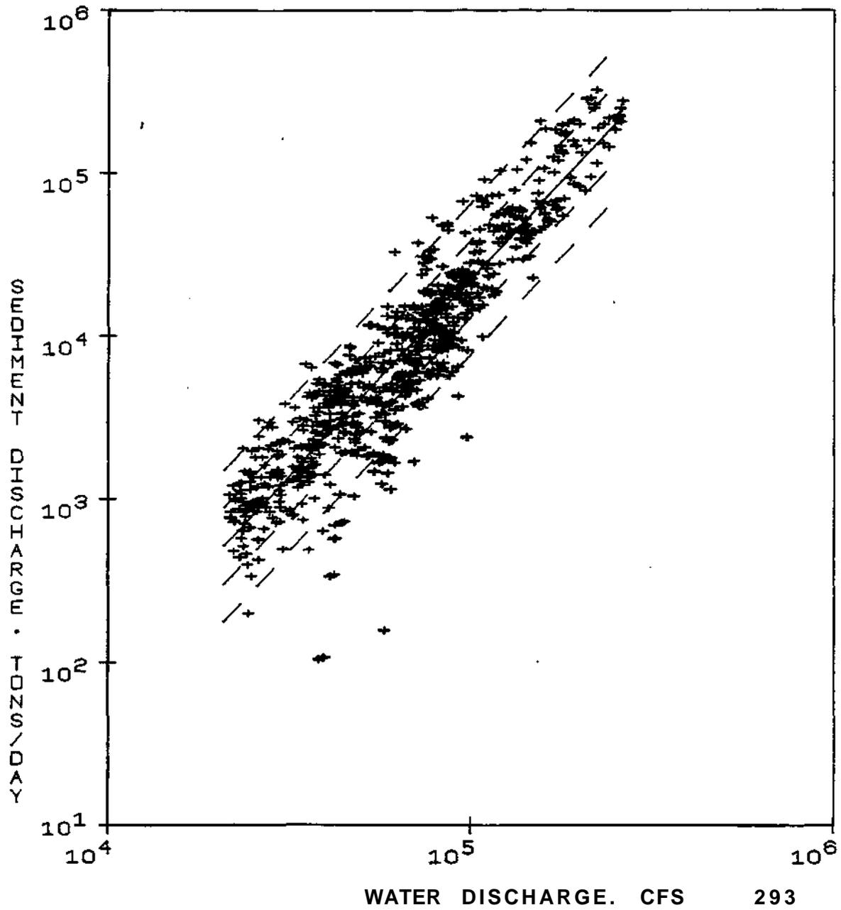
Figure 16. *Suspended sediment discharge versus water discharge for Mississippi River at Keokuk, Iowa*
