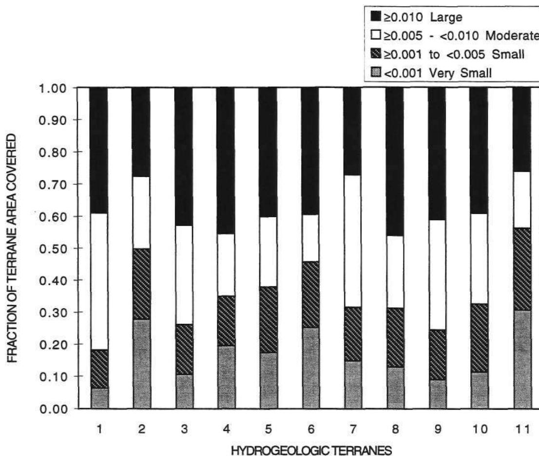
Figure 9. Distribution of watershed low-flow values for Illinois hydrogeologic terranes
