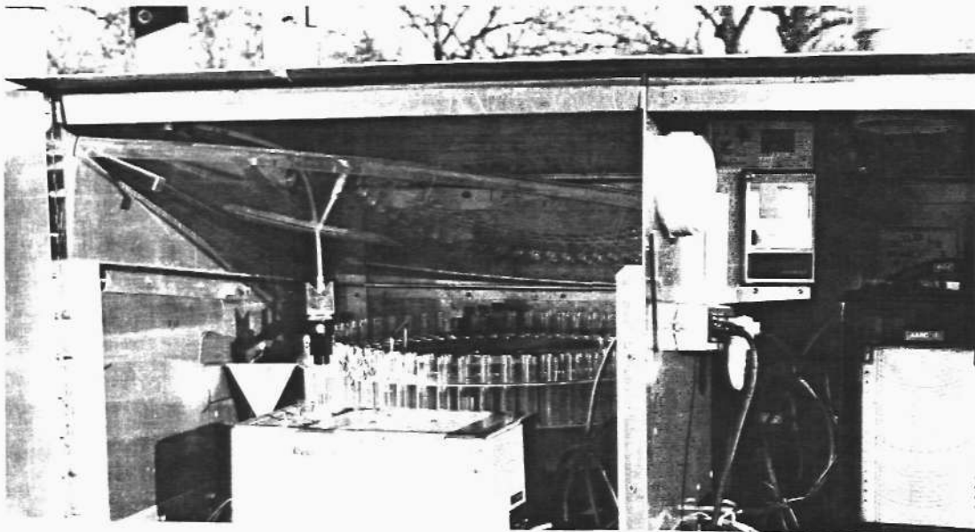
Figure 9-10. Water Survey scientists and technicians developed a series of sequential rainwater samplers over a 30-year period to measure how rainwater impurities shifted during a rain storm. Top is the first sampler, designed to be field operated with pulleys. Later models (below) operated with electrical power and employed smaller sampler bottles.
