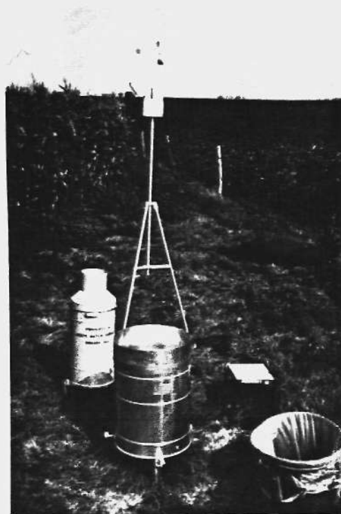
Figure 3-3. Field station #136 in the Central Illinois Network during 1970 showing (l.to r.) a weighing-bucket recording raingage, a Survey designed and built recording hailgage, an anemometer (behind the hailgage), a hail pad, and a plastic rainwater collector. The hail pad was a one square foot foam block (1-inch thick) covered with aluminum foil and it recorded as dents any hailstones that fell.
