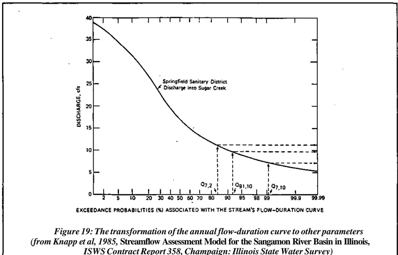
*Figure 19: The transformation of the annual flow-duration curve to other parameters (from Knapp et al, 1985, Streamflow Assessment Model for the Sangamon River Basin in Illinois, ISWS Contract Report 358, Champaign: Illinois State Water Survey)*
