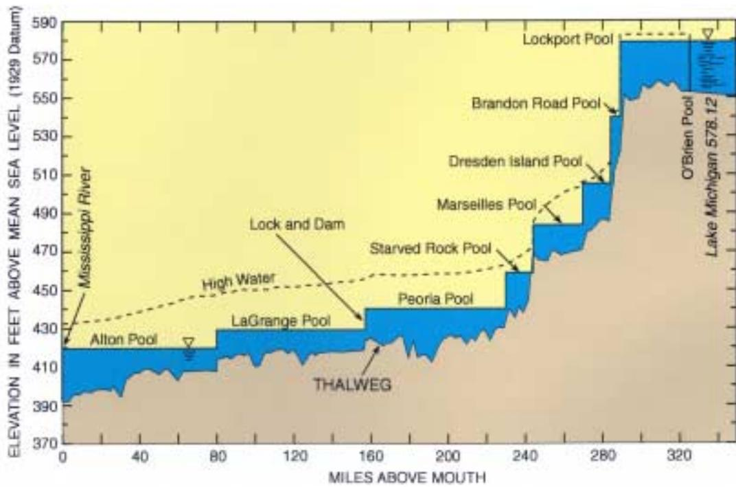
Figure 2. Profile of Illinois River Waterway.
