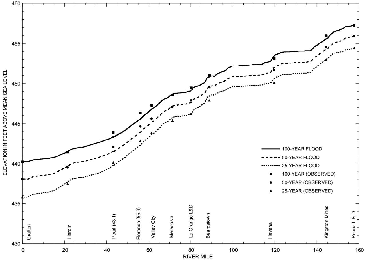
Figure 6. Simulated flood profiles for the Lower Illinois River with flood elevations for 25-, 50-, and 100-year flood events (4%, 2%, and 1% exceedence probability, respectively).
