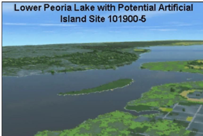
Figure 12. Still image from Lower Peoria Lake animation depicting proposed artificial island construction across from downtown Peoria's riverfront (upper left) and looking northeast. The island will be built with dredged material from the lake, as described in Demissie, Soong, and Bhowmik (1988).
