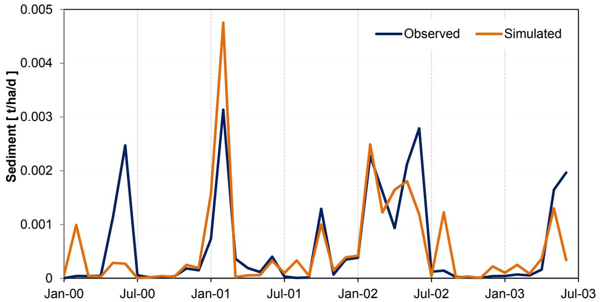
**Figure 2.10** Observed and simulated monthly sediment for Big Ditch watershed
