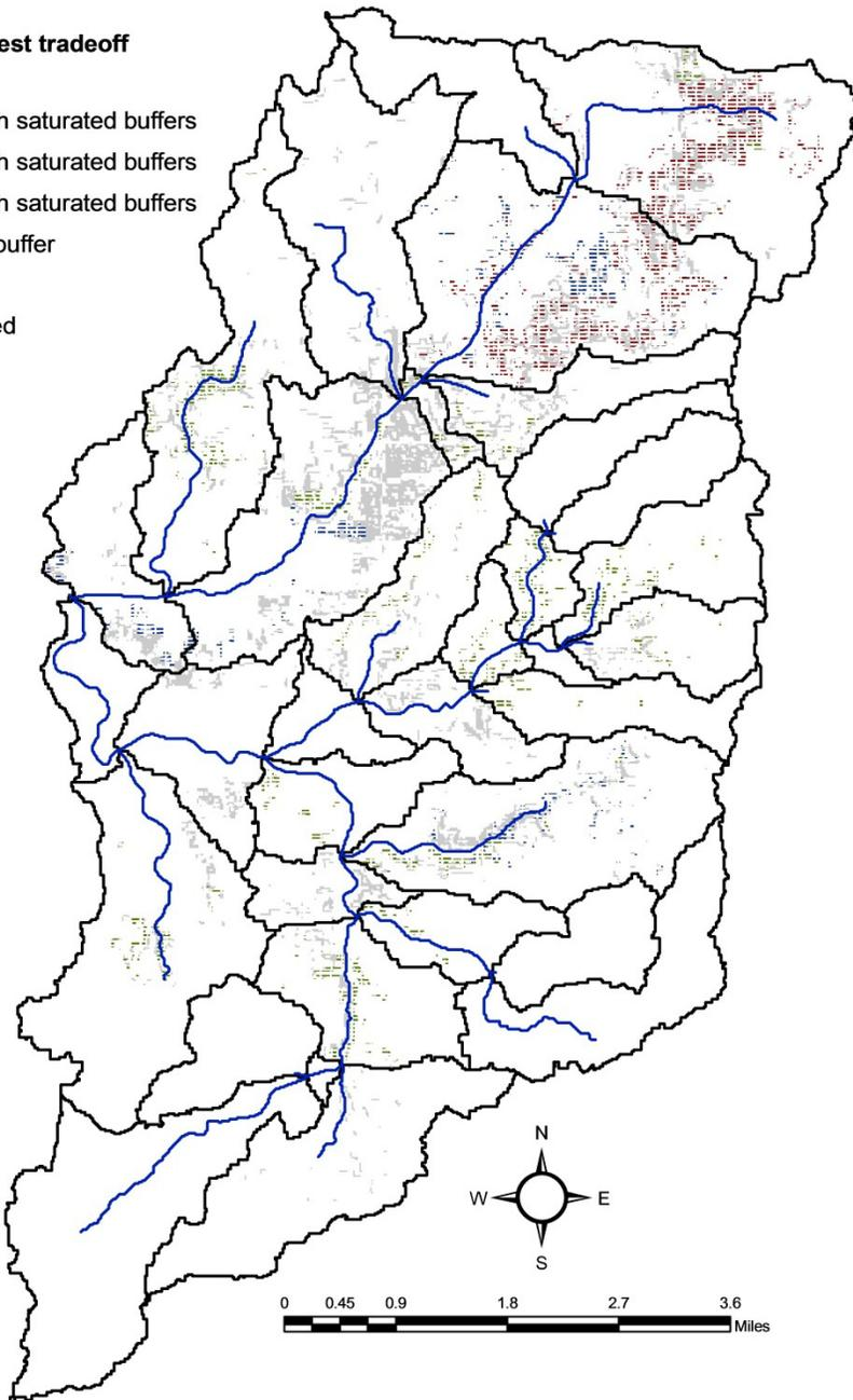
**Figure C.8 Optimal placement of saturated buffers in Big/Long Creek Watershed**
