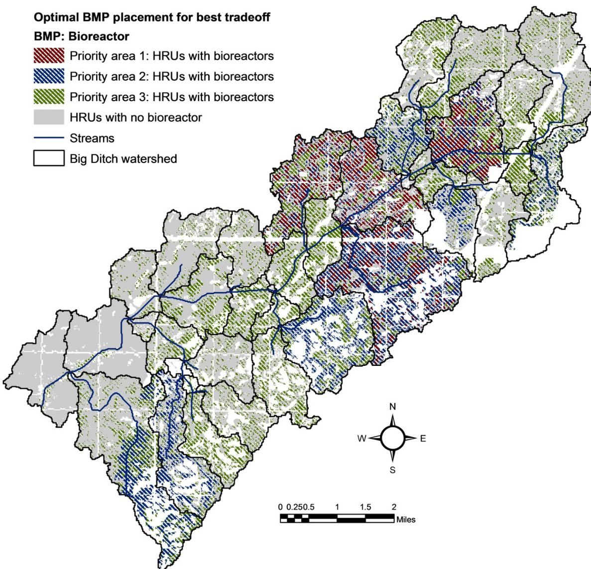
**Figure B.7** Optimal placement of bioreactors in Big Ditch Watershed
