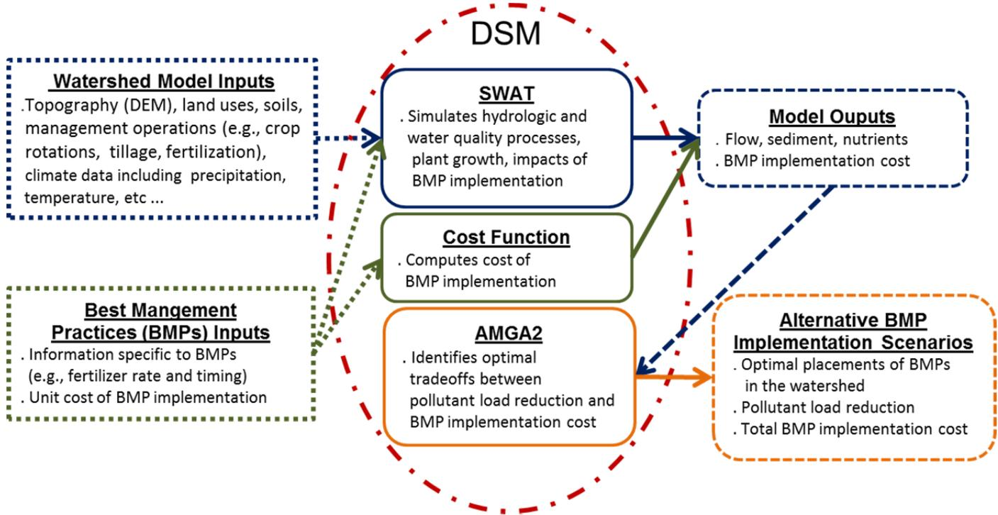
**Figure 4.1** Solution framework of the Decision Support Model (DSM)
