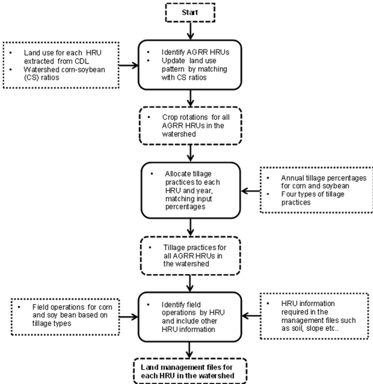
**Figure 2.8** Flow diagram used in preparation of land management files for the watershed models
