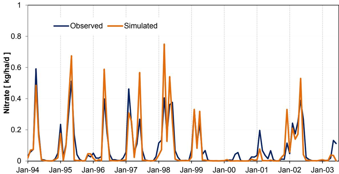
**Figure 2.11** Observed and simulated monthly nitrate for Big Ditch watershed
