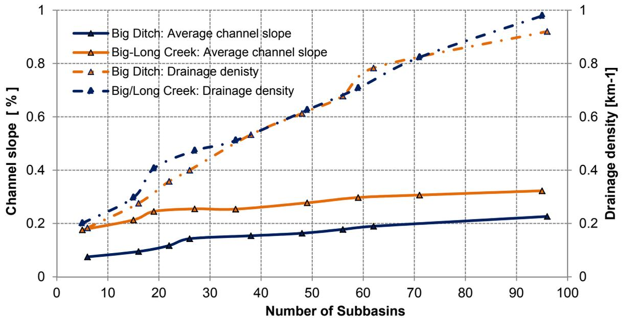
Figure 2.4 Effect of watershed subdivision levels on subbasin average channel slope and drainage density
