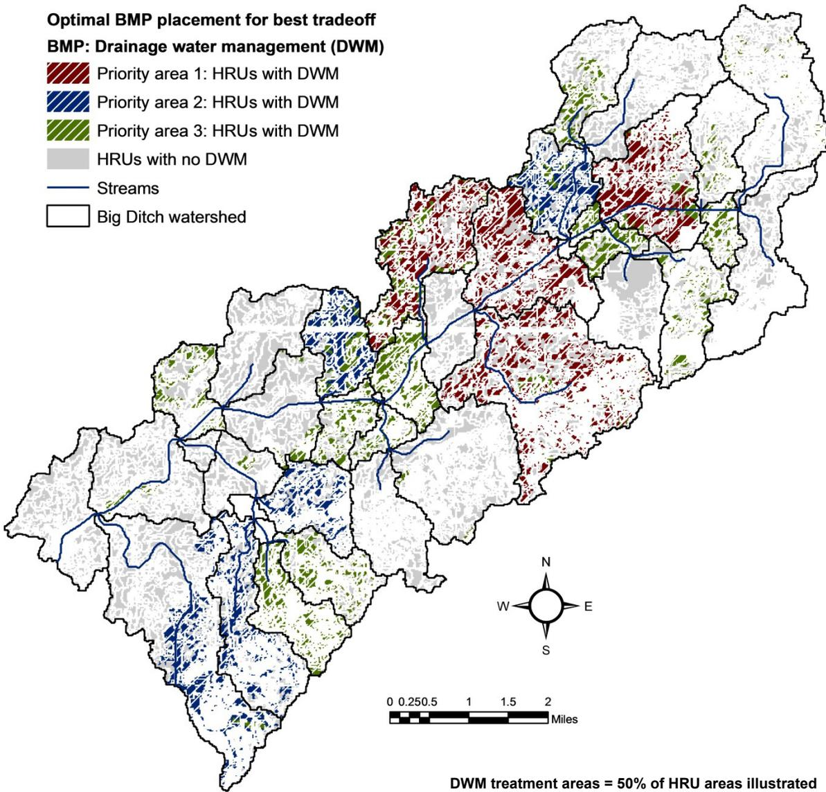
**Figure B.6** Optimal placement of drainage water management in Big Ditch Watershed
