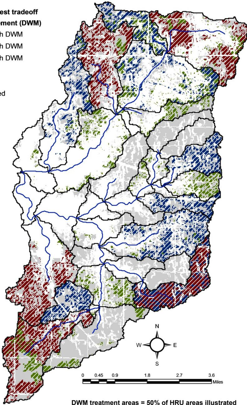
**Figure C.6** Optimal placement of drainage water management in Big/Long Creek Watershed
