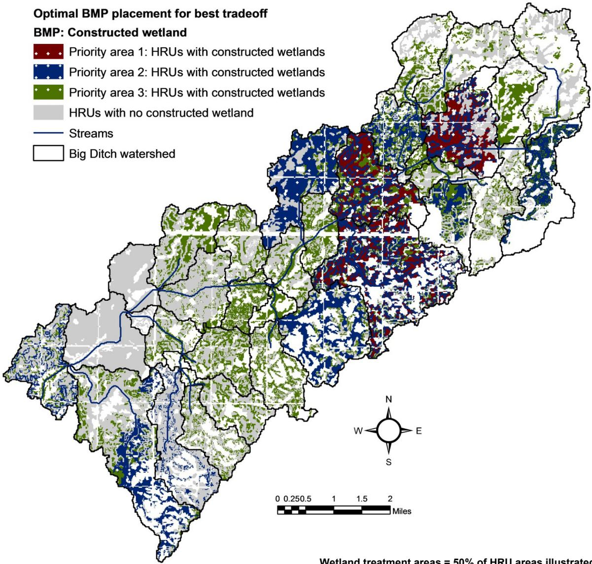
**Figure 4.12** Optimal placement of constructed wetlands in Big Ditch watershed
