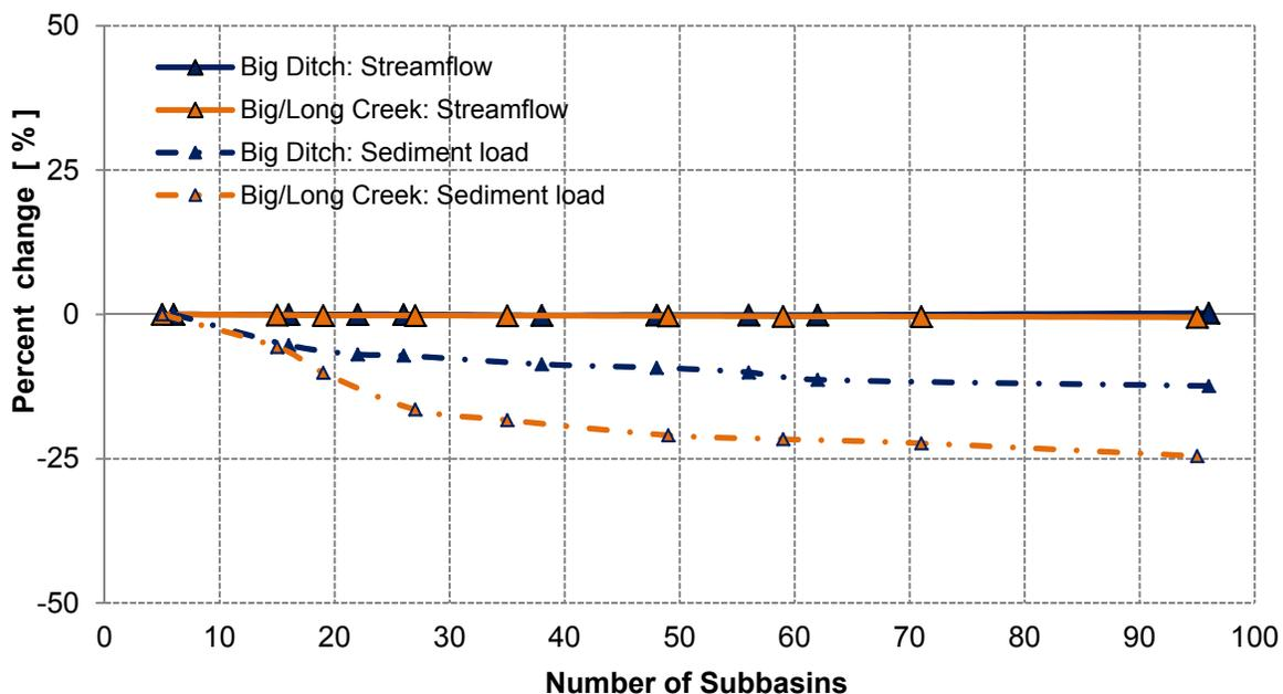
**Figure 2.5** Effect of watershed subdivision levels on average streamflows and sediment loads at the watershed outlets
