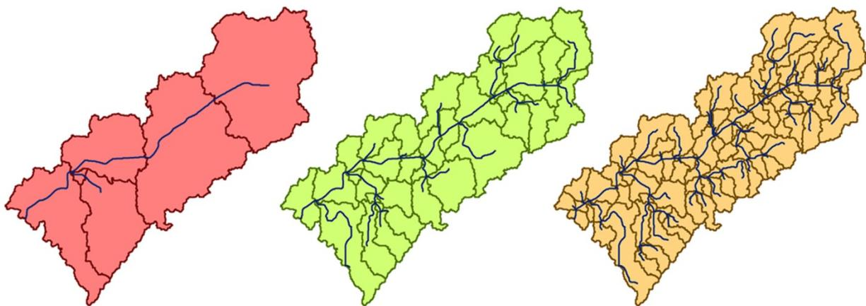
**Figure 2.2** Coarse, intermediate, and fine delineations for Big Ditch watershed
