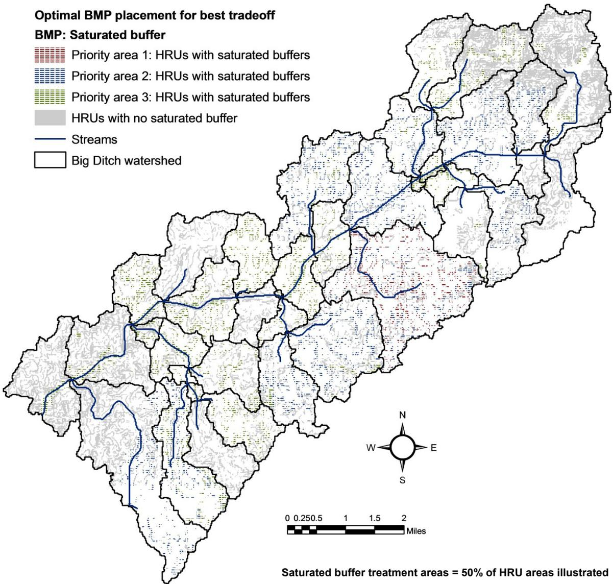
**Figure B.8** Optimal placement of saturated buffers in Big Ditch Watershed
