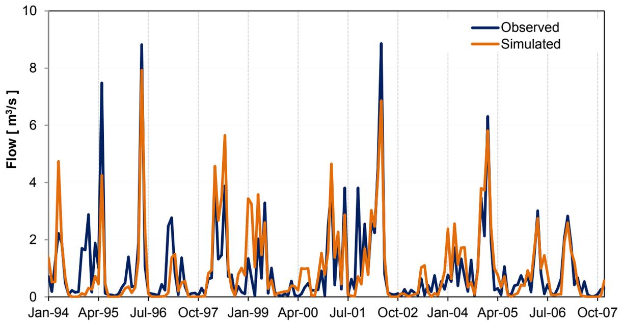
Figure 2.13 Observed and simulated monthly sediment for Big/Long Creek watershed
