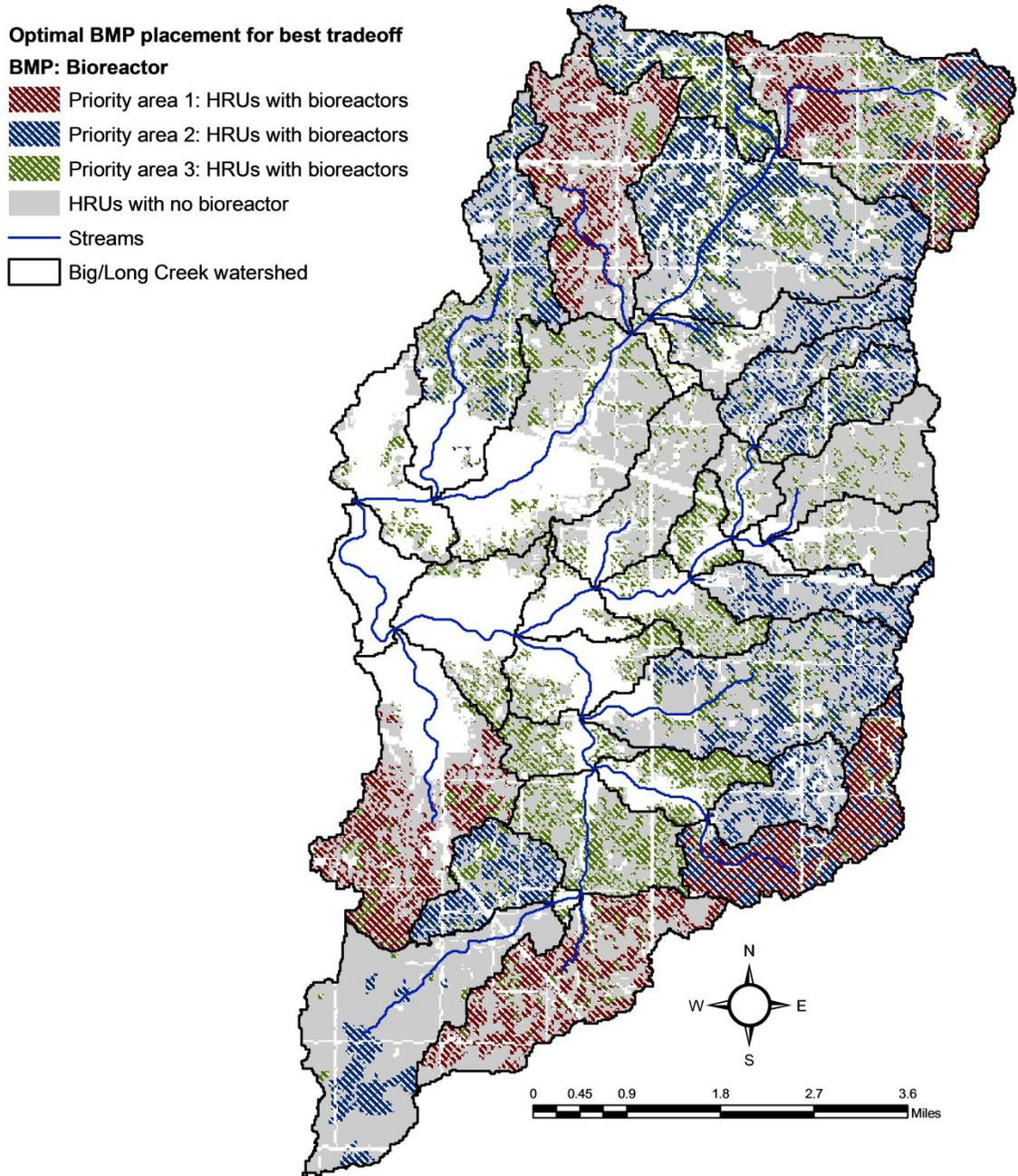
**Figure C.7** Optimal placement of bioreactors in Big/Long Creek Watershed
