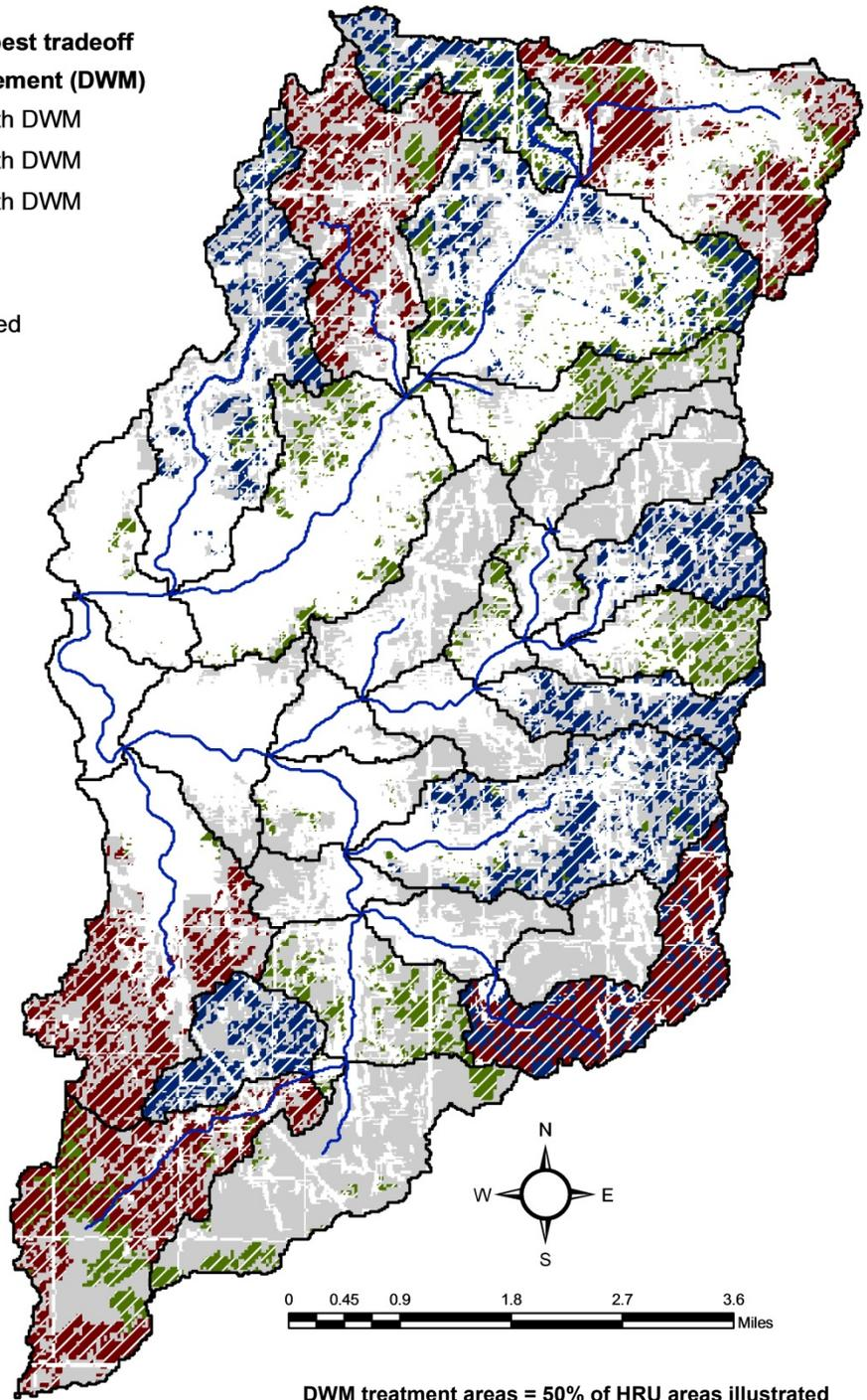
**Figure 4.14** Optimal placement of drainage water management in Big/Long Creek watershed
