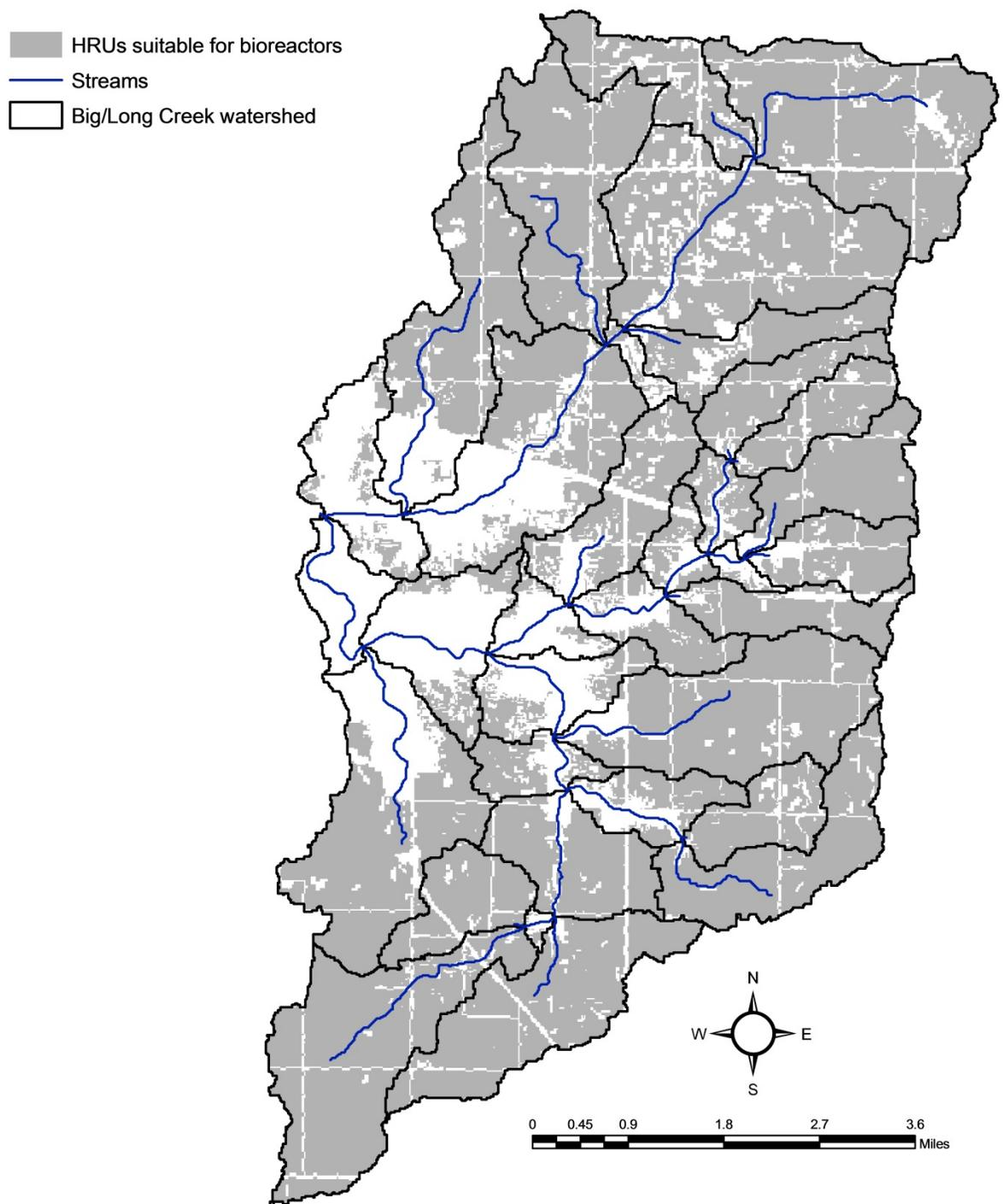
**Figure A.8** Big/Long Creek HRUs suitable for bioreactors
