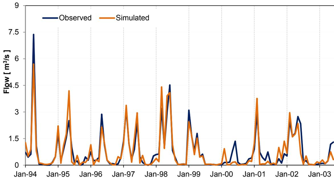
**Figure 2.9** Observed and simulated monthly flow for Big Ditch watershed
