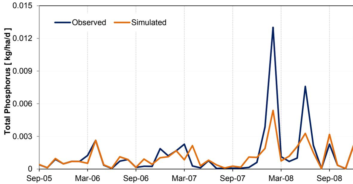
Figure 2.12 Observed and simulated monthly total phosphorus for Big Ditch watershed
