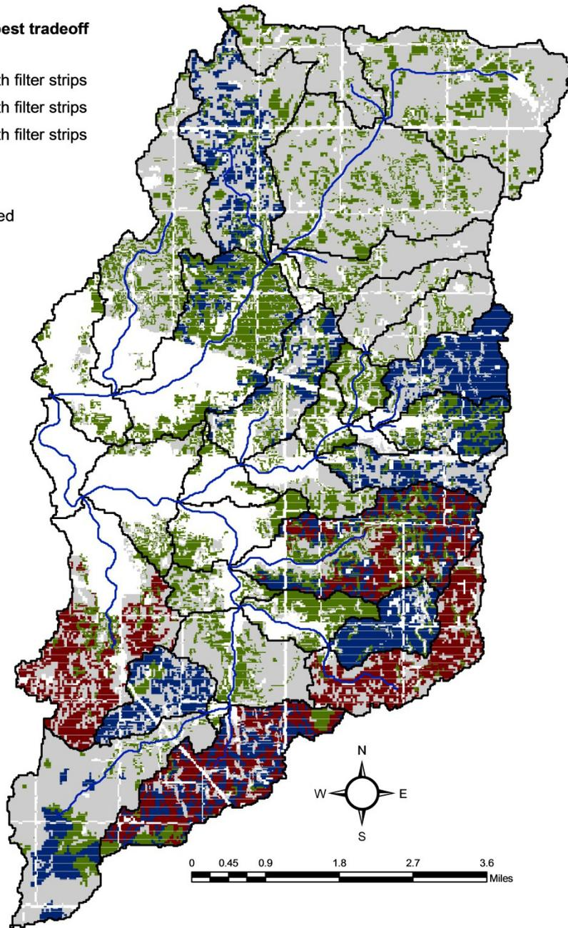
**Figure C.9** Optimal placement of filter strips in Big/Long Creek Watershed
