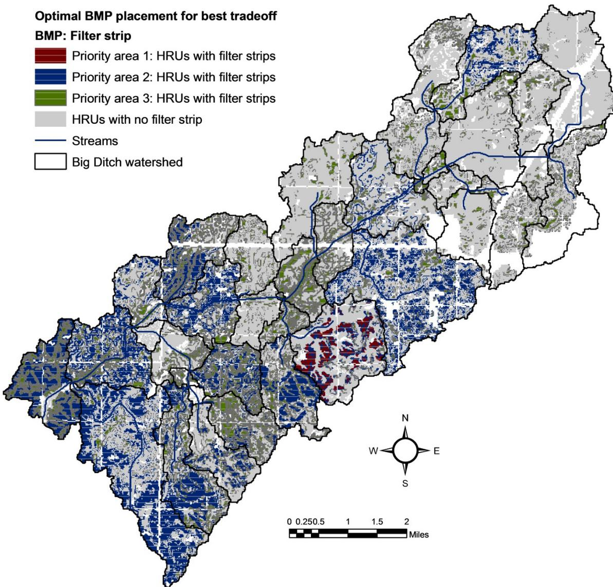
Figure 4.20 Optimal placement of filter strips in Big Ditch watershed
