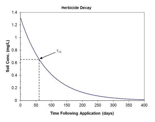
Figure 1. Idealized herbicide decay with the half-life indicated
