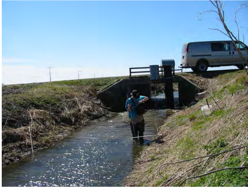
Figure 9. Measuring discharge upstream of stilling well, ISCO shelter and equipment shelter on Kickapoo Creek (Control [211])
