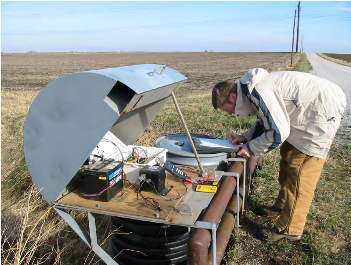
Figure 4. Typical streamgaging station and automatic pump water sampler
