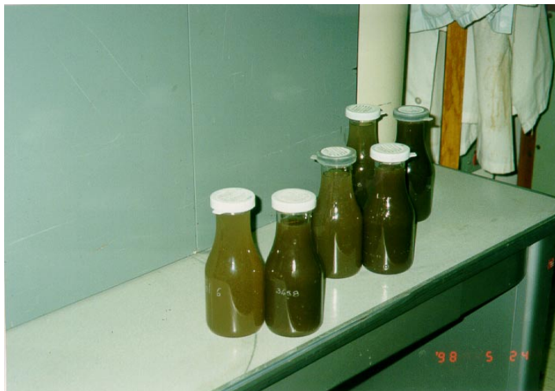
Figure 6b. Suspended sediment samples collected during an April storm in 1999. Similar to the explanation for Figure 6a, these samples were collected from sites 4, 1, and 3 (repeated for comparison purposes). Samples to the left in each pair were collected a day later. The printed year on the photo was entered incorrectly.
