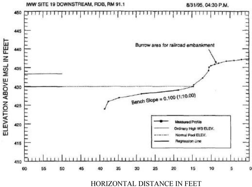
Figure 100. Bank sections at site 19 (concluded)
