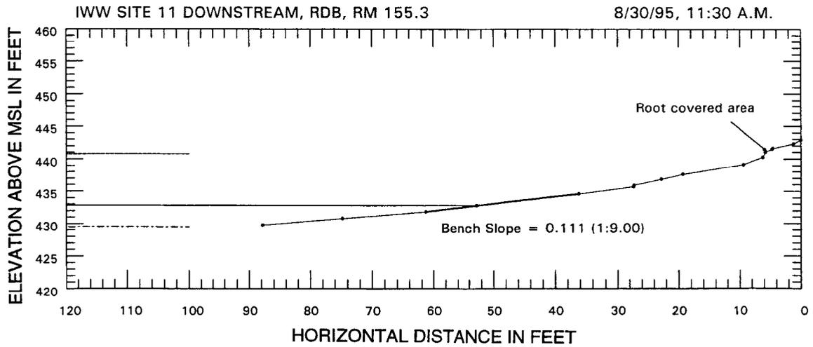
Figure 78. Bank sections at site 11 (concluded)
