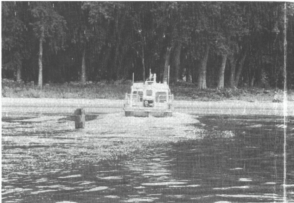
Figure 7. River cross-section measurement by an ISWS boat equipped with GPS and sonar
