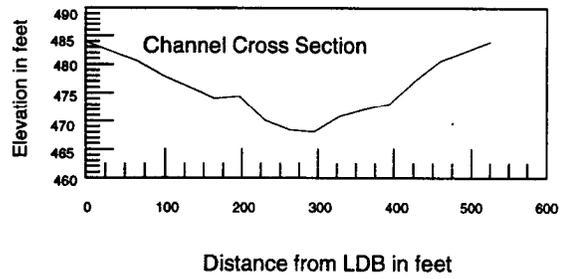
Figure 38. Bank sections at site UP1
