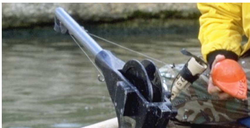
Figure 22. Downrigger fitted with YSI DO/temperature meter, stirrer, and probes
