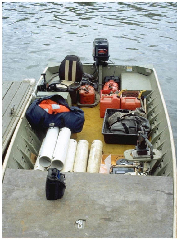
Figure 18. Boat with monitors in protective shrouds
