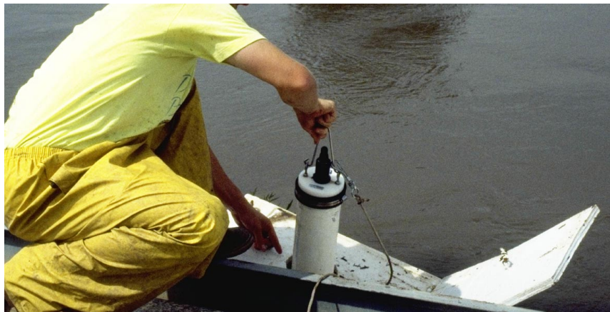
Figure 15. Inserting Data Sonde I into type III rigging
