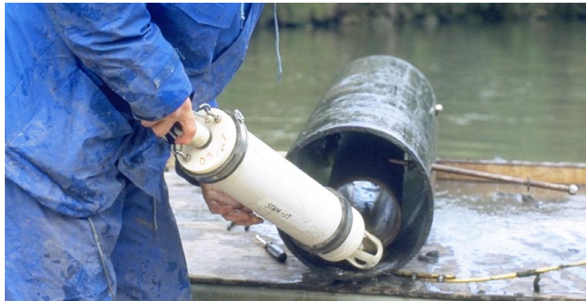
Figure 20. Exchanging a DataSonde I monitor at a type IA site
