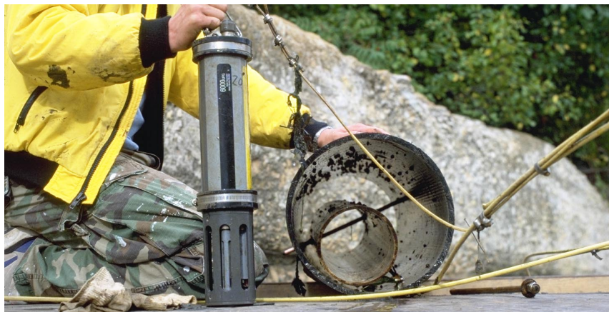
Figure 21. Exchanging a YSI 6000 monitor at a type IA site
