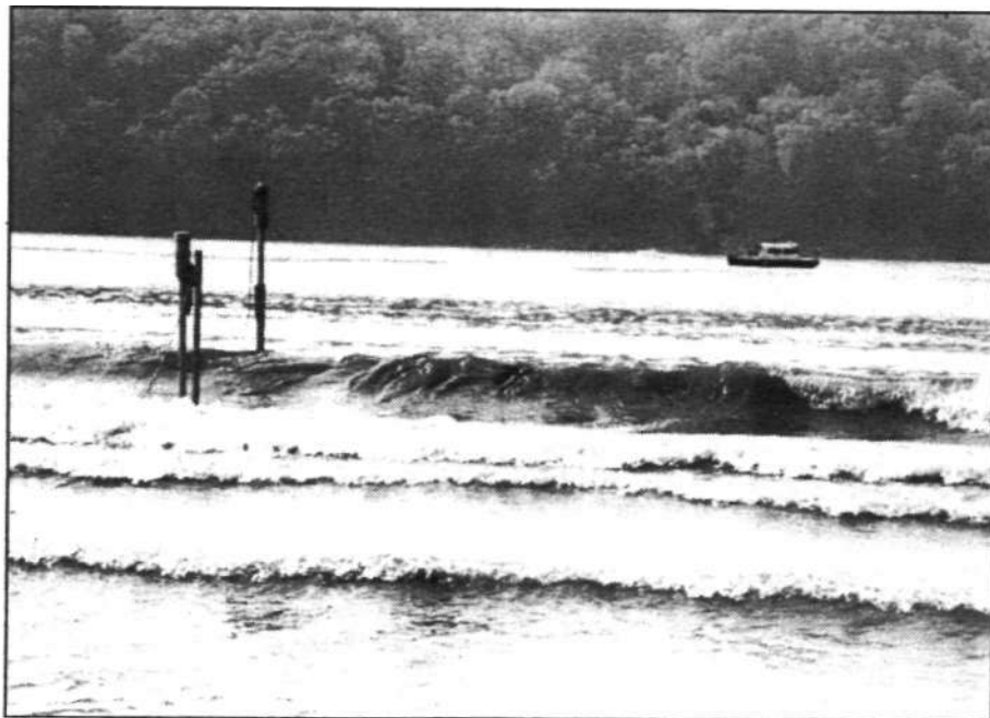
Figure 9. Tow-induced waves at the wave gages
