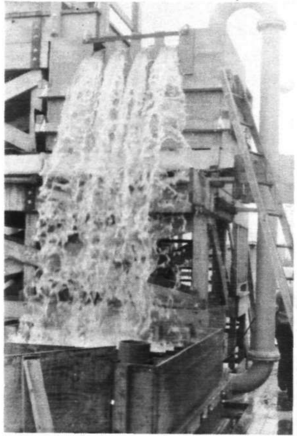
Front view of four-partition, 10-foot free-fall weir at high flow
