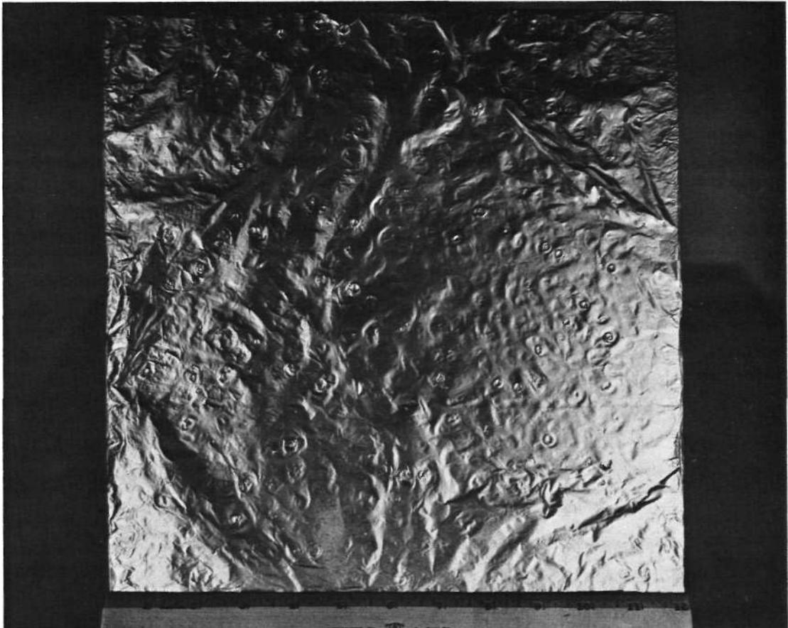
Fig. 6b Imprint of clear, hard hail registered after long term (8 day) exposure of indicator.
