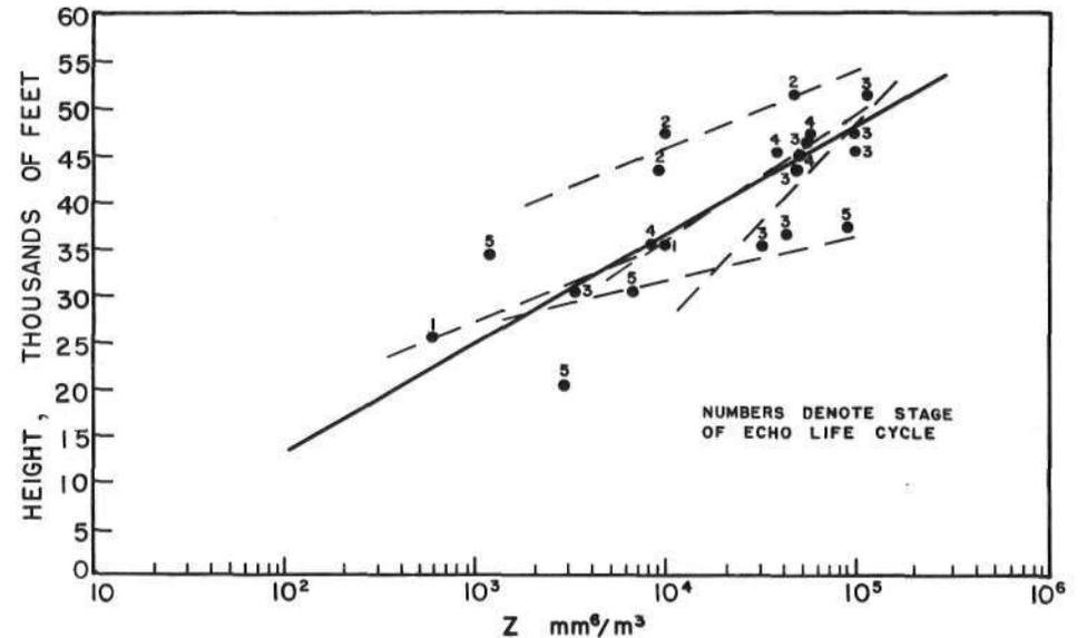
Fig. 11 Radar reflectivity ( $Z$ ) vs. height, September 28, 1959.
