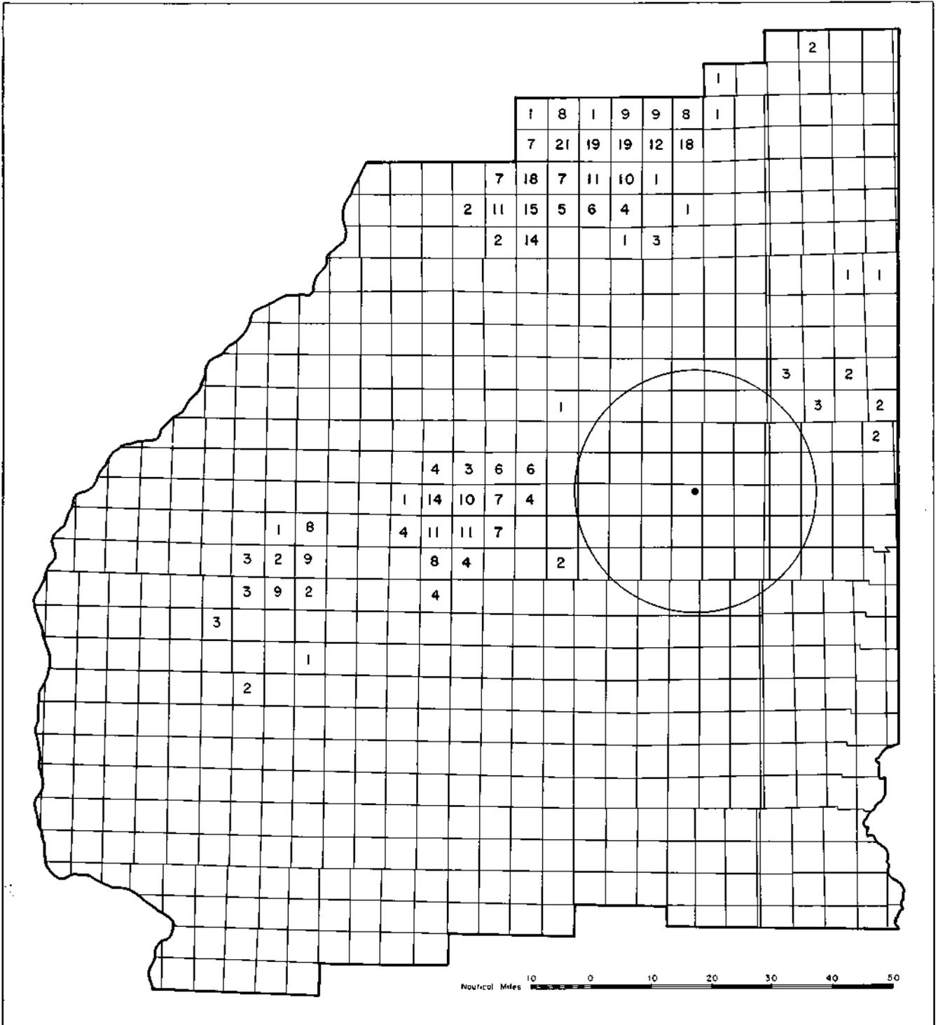
Fig. 14 Total radar reflectivity factor (Z) x 10<sup>4</sup>mm<sup>6</sup>m<sup>-3</sup> at 20,000 feet based on 9-minute observations for hail period, September 28, 1959.
