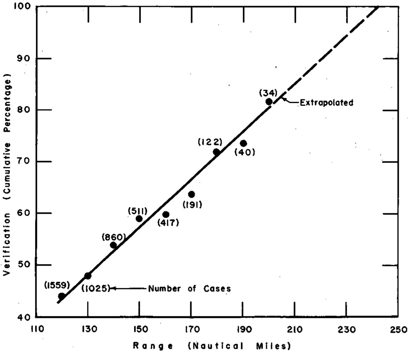
Fig. 1 Verification of hail occurrences vs. radar echo range (after Cook).
