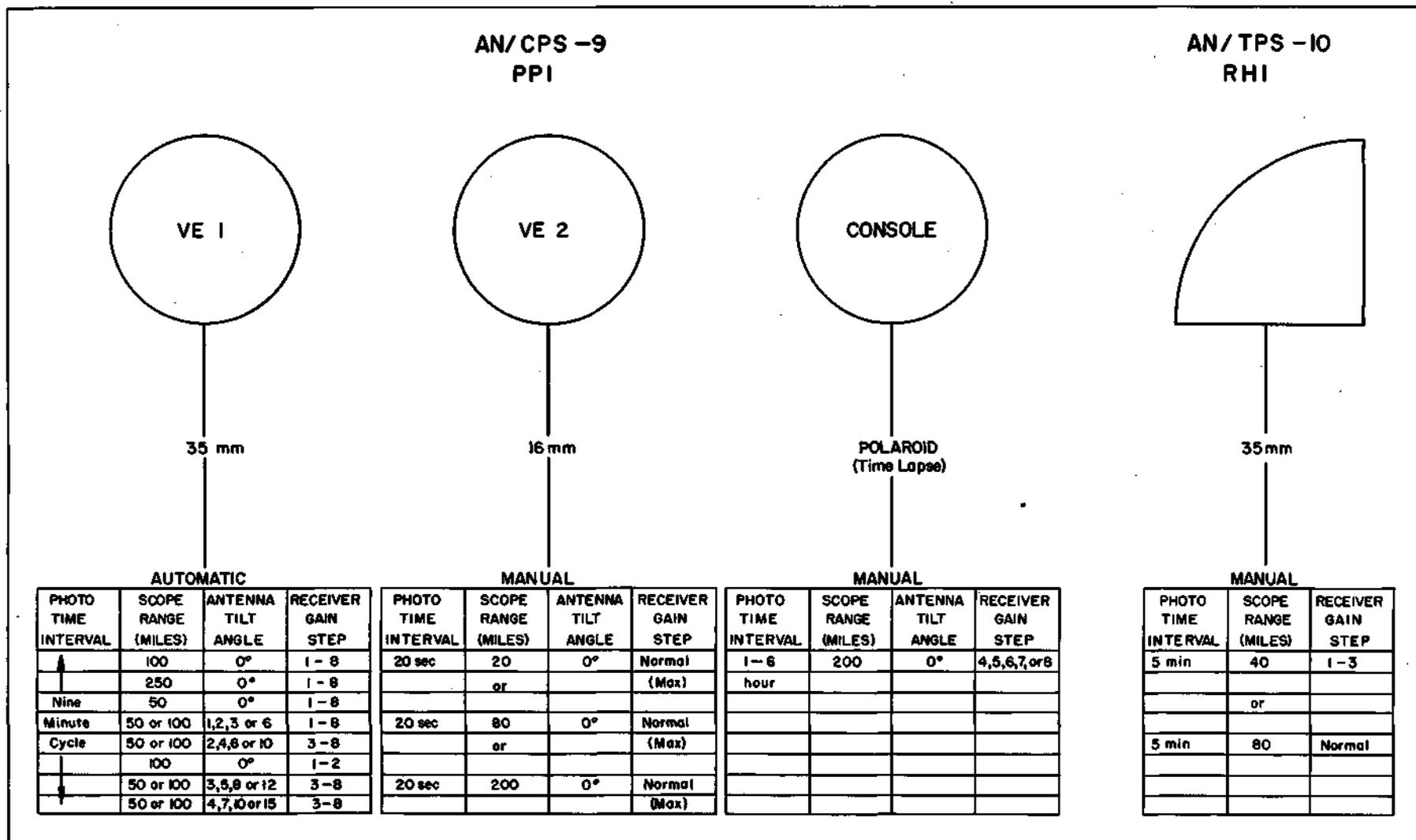
Fig. 2 Radar data recording schematic.
