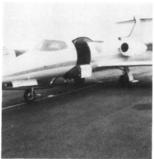
Flare container built in bottom of modified Lear jet used to drop flares for hail suppression in South Africa
