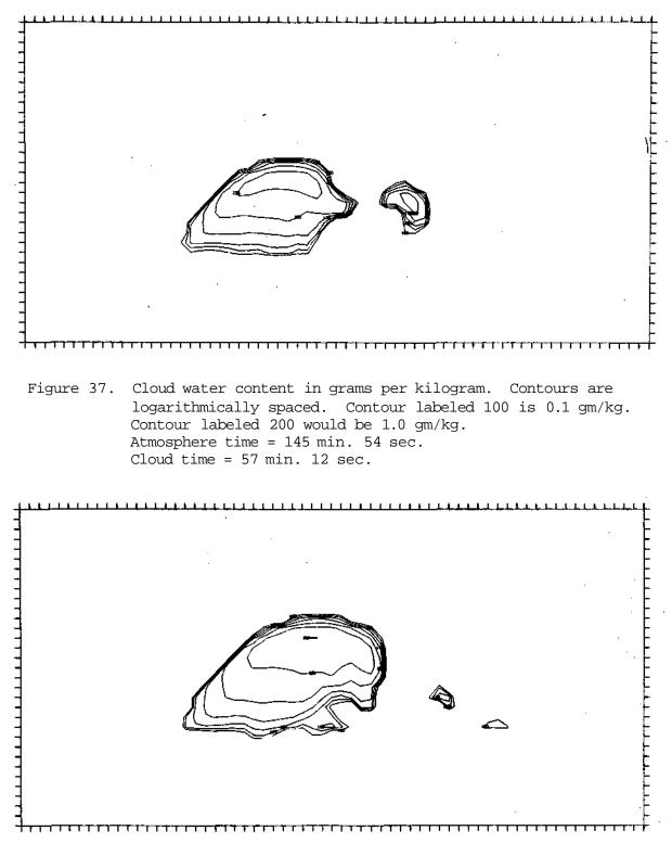
Figure 38. Cloud water content in grams per kilogram. Contours are logarithmically spaced. Contour labeled 100 is 0.1 gm/kg. Contour labeled 200 would be 1.0 gm/kg. Atmosphere time = 151 min. 54 sec. Cloud time = 63 min. 12 sec.
