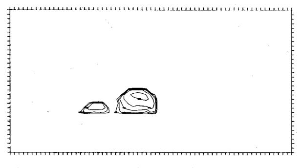
Figure 34. Cloud water content is grams per kilogram. Contours are logarithmically spaced. Contour labeled 100 is 0.1 gm/kg. Contour labeled 200 would be 1.0 gm/kg. Atmosphere time = 131 min. 54 sec. Cloud time = 43 min. 12 sec.
