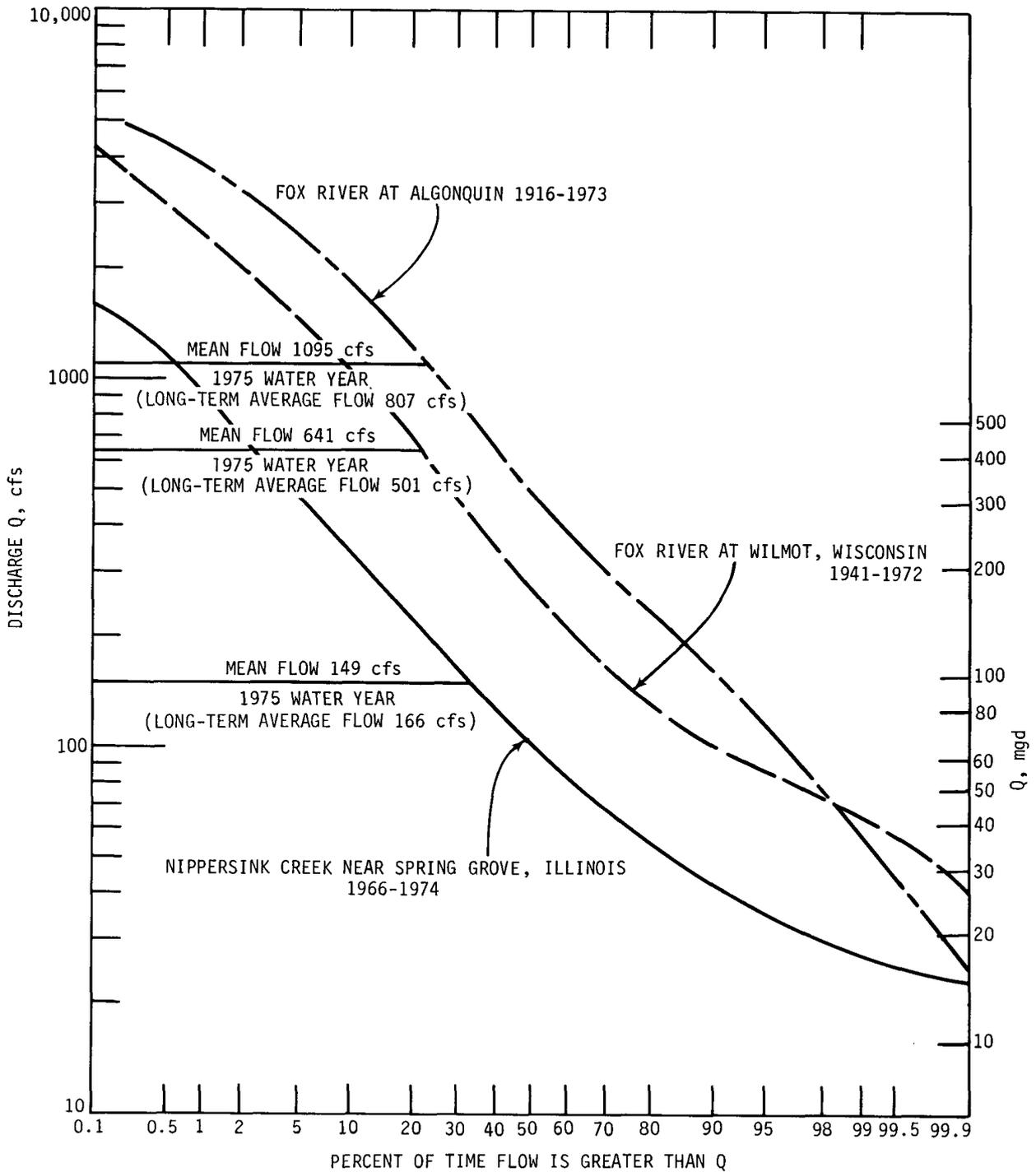
Figure 36. Flow duration curves for gaging stations in Chain of Lakes region
