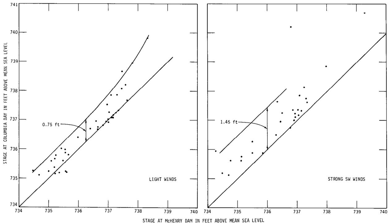
Figure 15. Stage variations between Columbia Bay and McHenry Lock and Dam for different wind conditions
