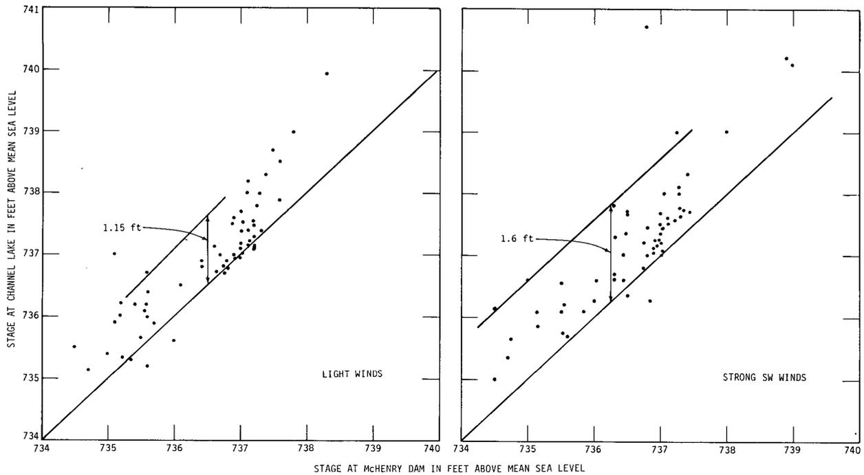
Figure 16. Stage variations between Channel Lake and McHenry Lock and Dam for different wind conditions
