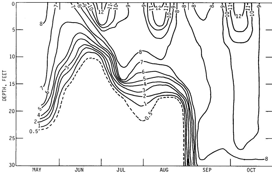
Figure 94. Isoleths of dissolved oxygen in Pistakee Bay
