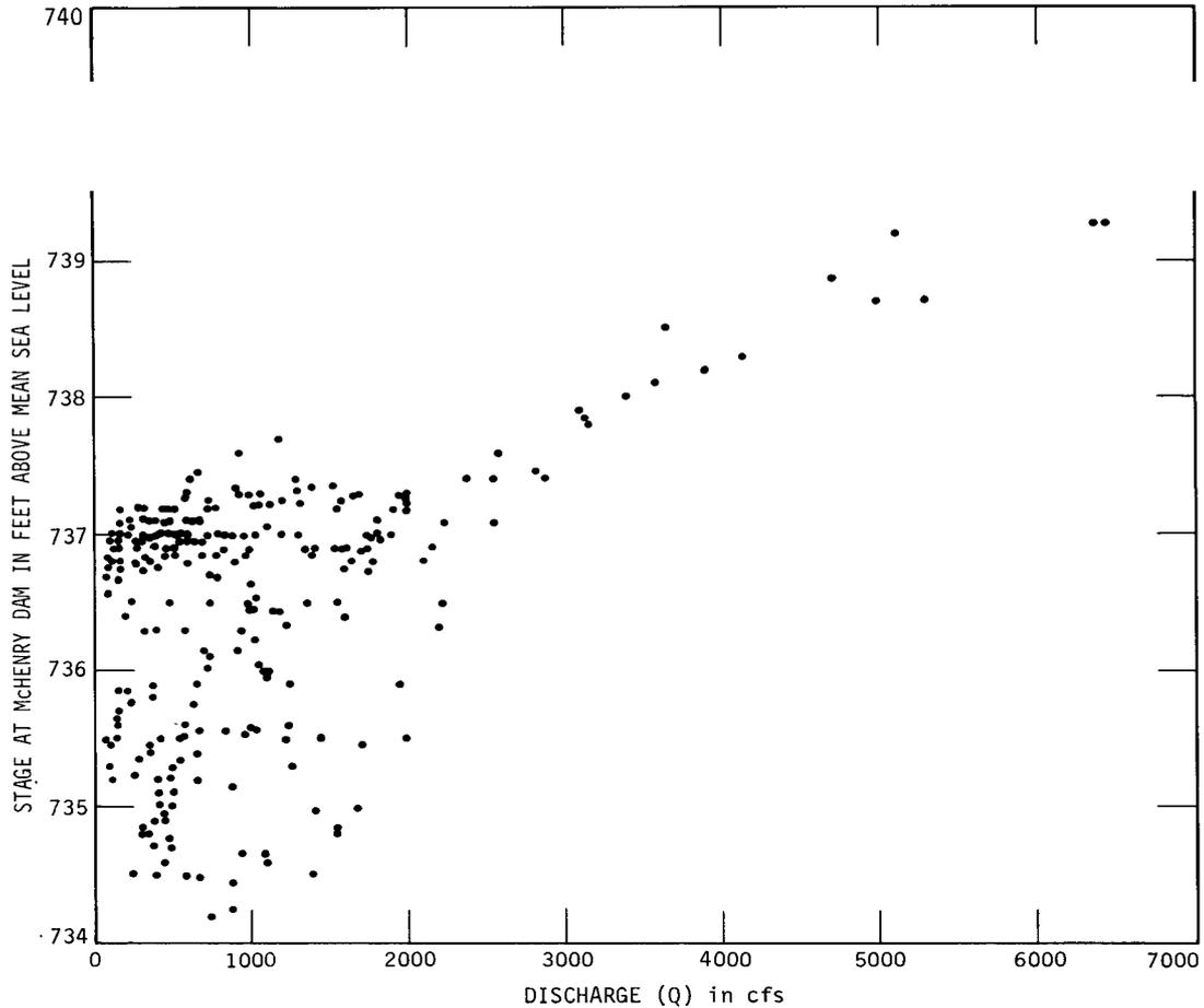
Figure 20. Stage versus discharge at McHenry Dam (1959-1974)
