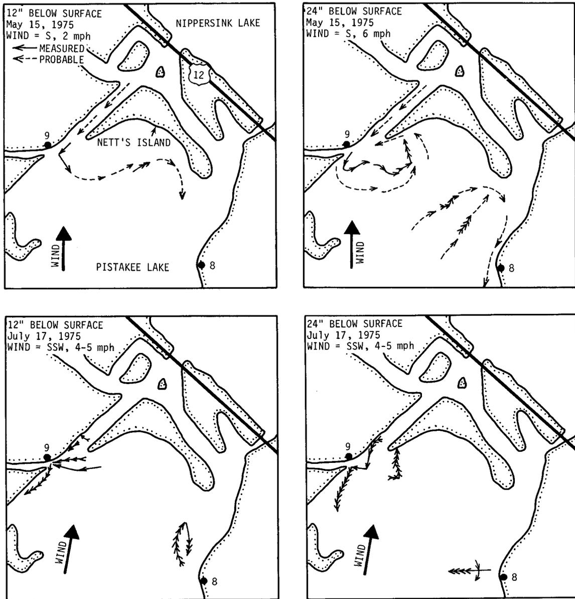
Figure 58. Flow pattern downstream of Highway 12 Bridge for May 15 and July 17, 1975
