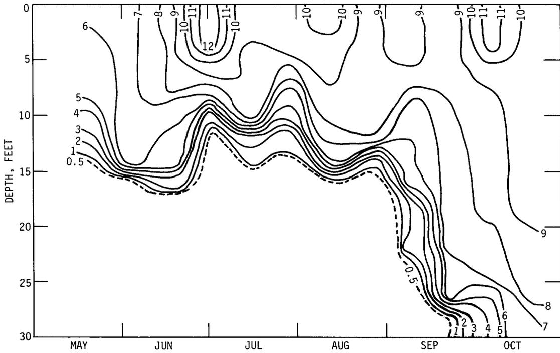
Figure 92. Isoleths of dissolved oxygen in Bluff Lake
