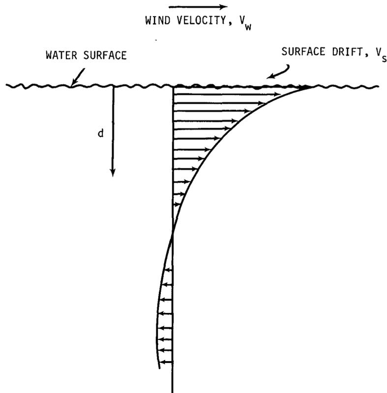
Figure 45. Schematic of surface drift and flow profile
