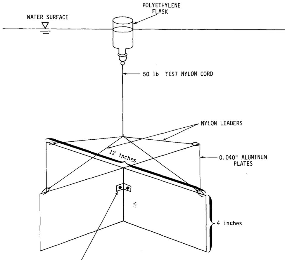
Figure 22. Float and cross-vane used to measure circulation patterns
