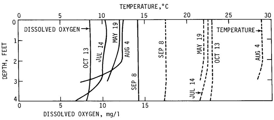
Figure 88. Temperature and dissolved oxygen profiles in Grass Lake (south)
