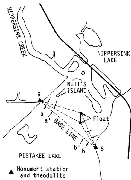
Figure 23. Schematic of circulation data collection
