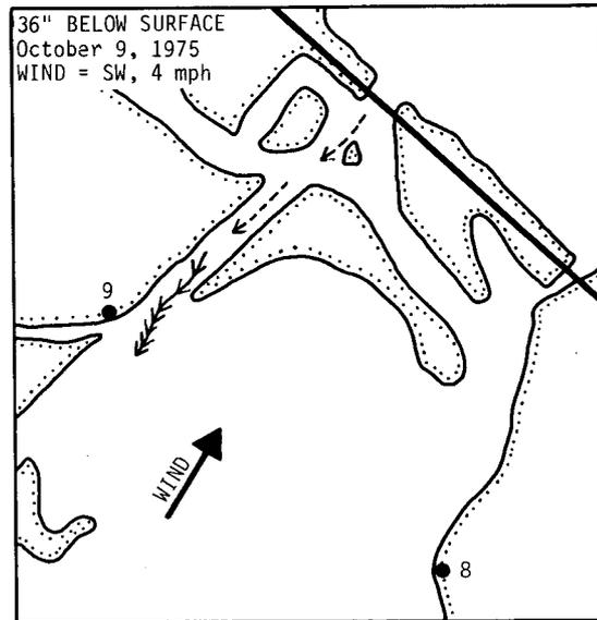
Figure 59. Flow pattern downstream of Highway 12 Bridge for October 9, 1975
