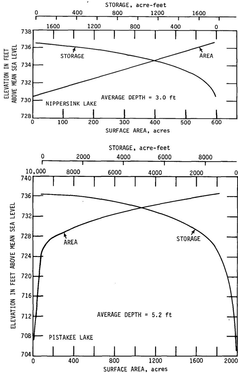
Figure 26. Depth-area and depth-storage relationships for Pistakee and Nippersink Lakes
