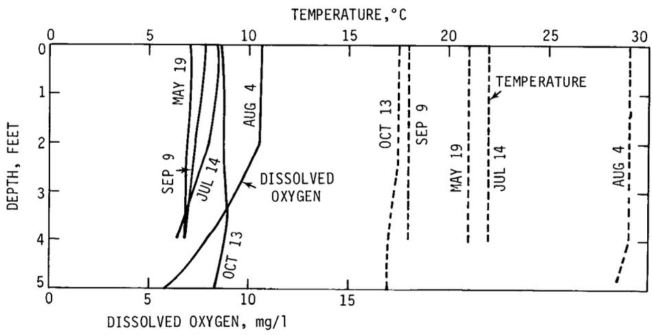
Figure 84. Temperature and dissolved oxygen profiles in Nippersink Lake
