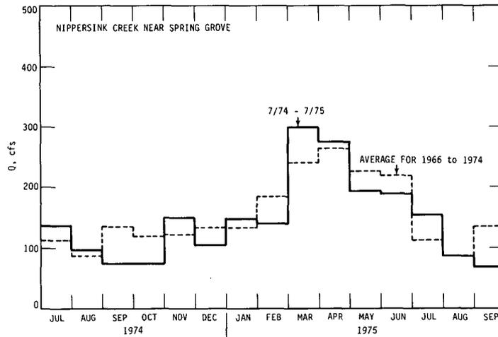
Figure 34. Monthly mean discharges for 1974-1975 and long-term mean discharges for Nippersink Creek near Spring Grove
