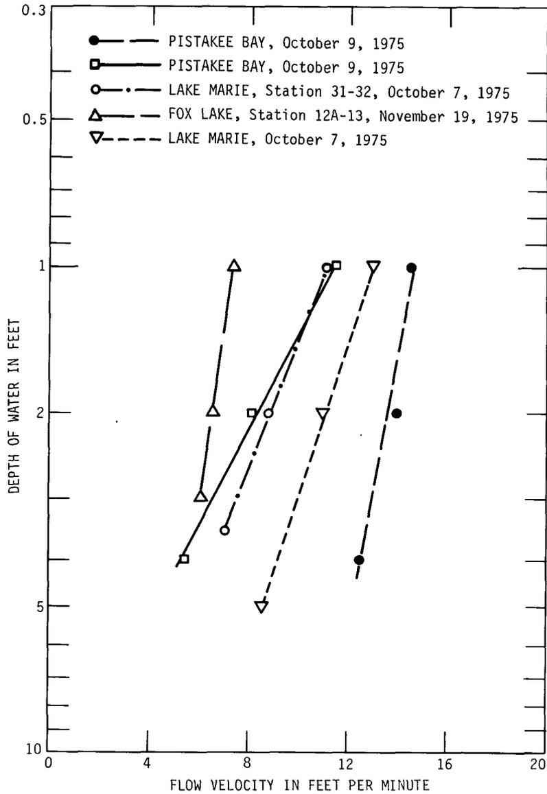
Figure 64. Typical vertical current profile (logarithmic)
