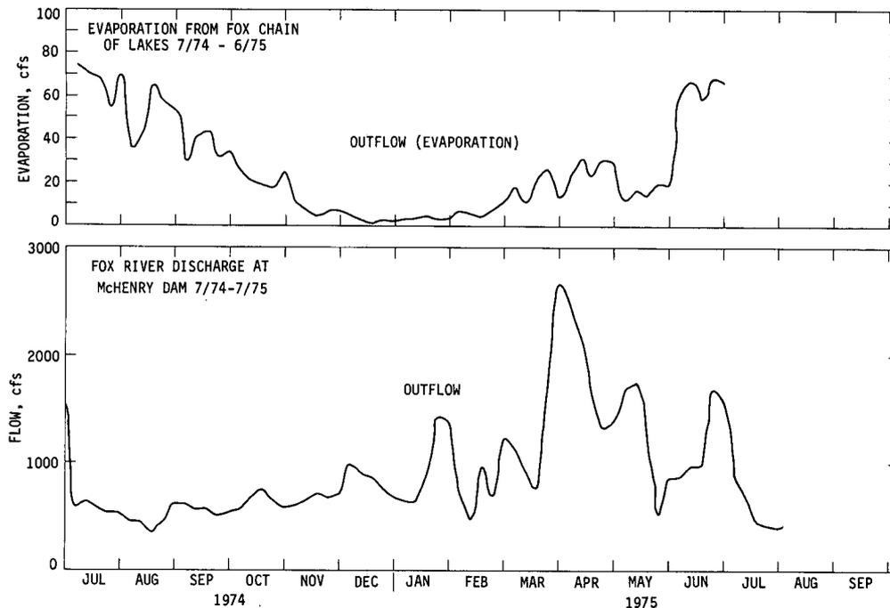
Figure 39. Evaporation losses for lakes and outflow at McHenry Dam
