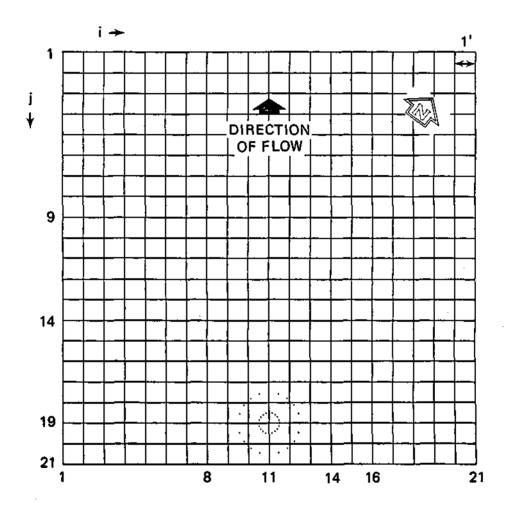
Figure 14. An example of particles plotted on a finite difference grid (see Naymik and Sievers, 1983).
