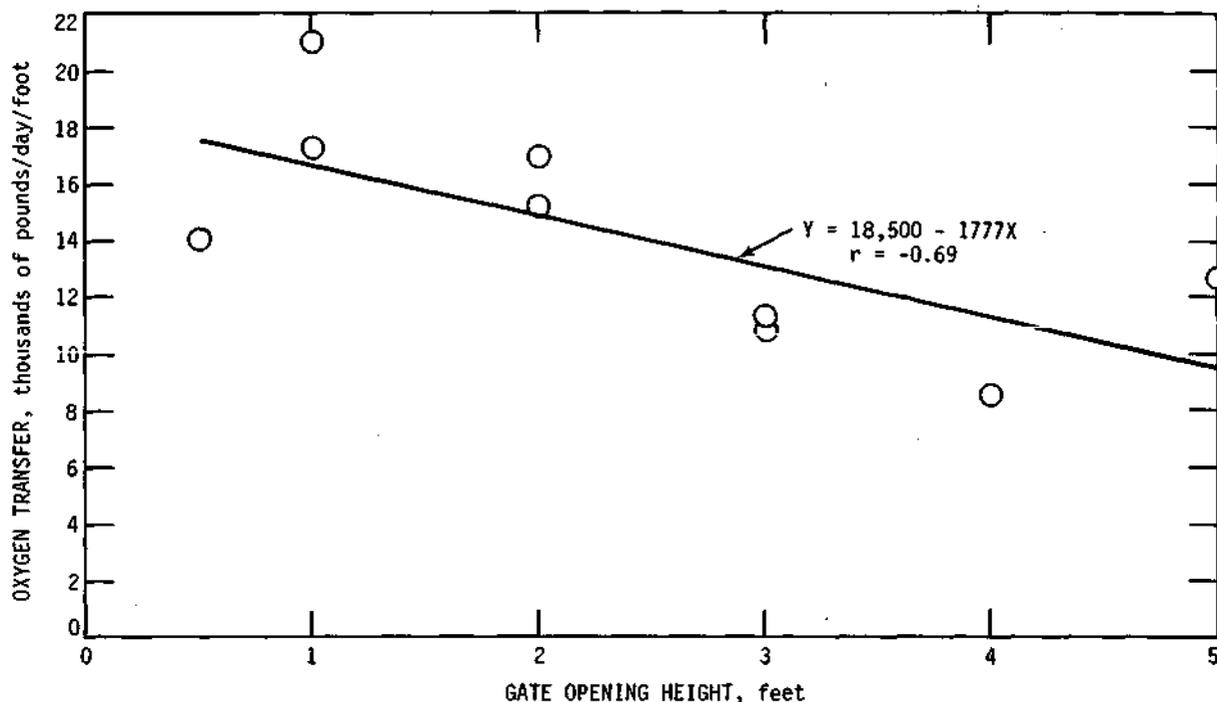
Figure 7. Dissolved oxygen Transfer rates for Marseilles Dam Tainter gate openings ( $C_A = 5 \text{ mg/l}$ ,  $T = 20^\circ\text{C}$ , Upper Pool Elev. 483.25, L.P. Elev. 471.0)
