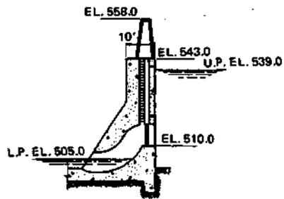
CROSS SECTION OF SLUICE GATE
