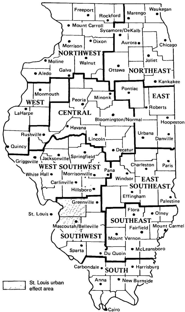
Figure 7. Precipitation-reporting stations and climatic sections used in developing Illinois frequency relations
