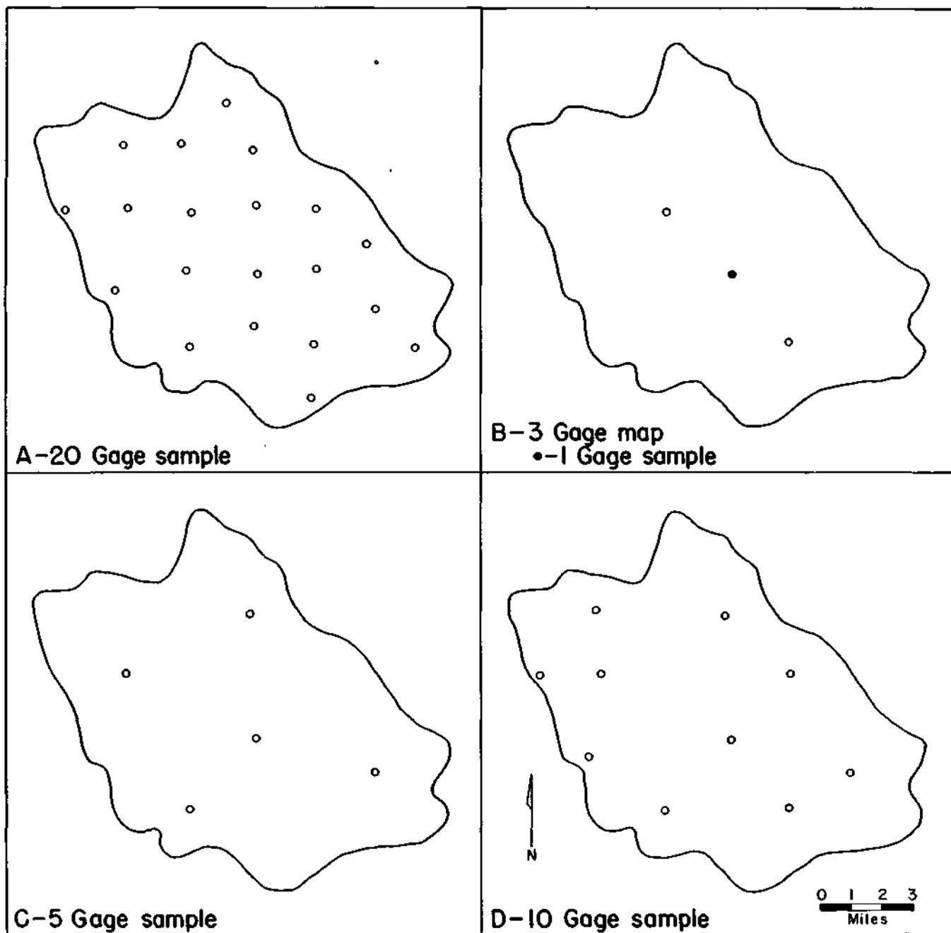
FIGURE 44 BEST-CENTERED SAMPLING PLAN FOR PANTHER CREEK NETWORK
