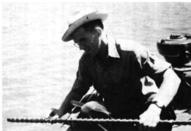
FIG. 4. USE OF SPUD IN MEASURING SEDIMENT THICKNESS.
