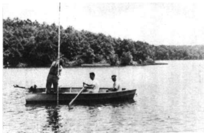
FIG. 5. USE OF SOUNDING POLE IN MEASURING SEDIMENT THICKNESS
