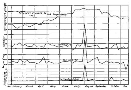
FIG. 12.—VARIATIONS IN EFFLUENT FROM CHAMBER B2, SECOND CHAMBER OF TANK B: CITY SEWAGE
